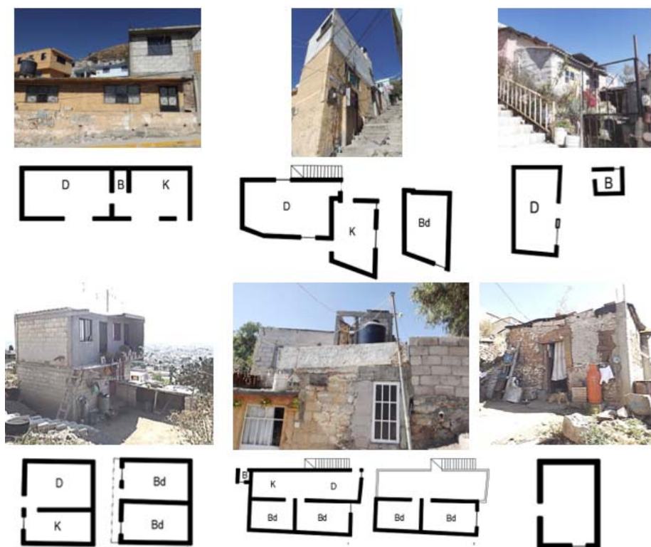
Figure 10. Examples of case studies. K (Kitchen), B (Bathroom), D (dining room), Bd (Bedroom).
