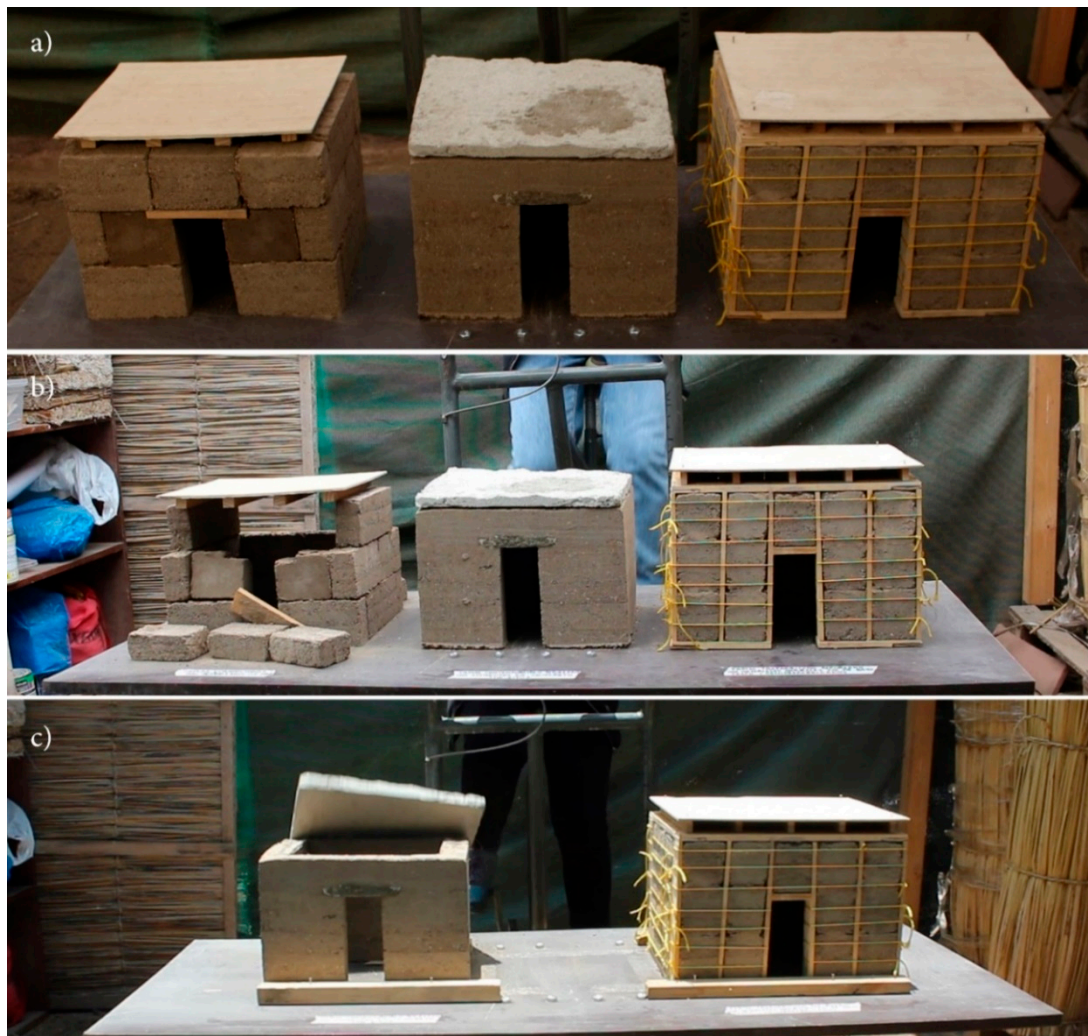
Figure 1. Phases of the qualitative dynamic comparative test: (a) the three models are placed on the shake table; (b) collapse of the unreinforced model; (c) better performance of our technology compared to concrete reinforced model.
