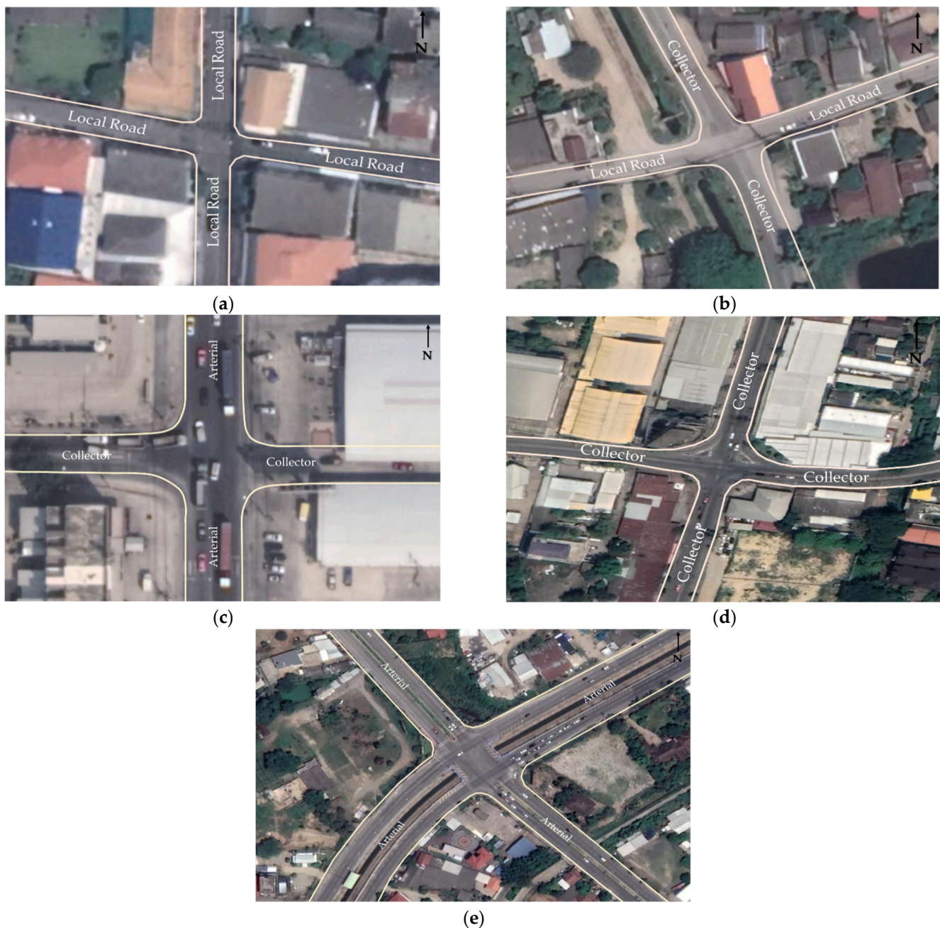
Figure 5. Layouts for five intersections of functionally classified roadways: (a) Local-road/Local-road; (b) Local/Collector; (c) Collector/Arterial; (d) Collector/Collector; and (e) Arterial/Arterial. Pictures were taken from Google Street View.
