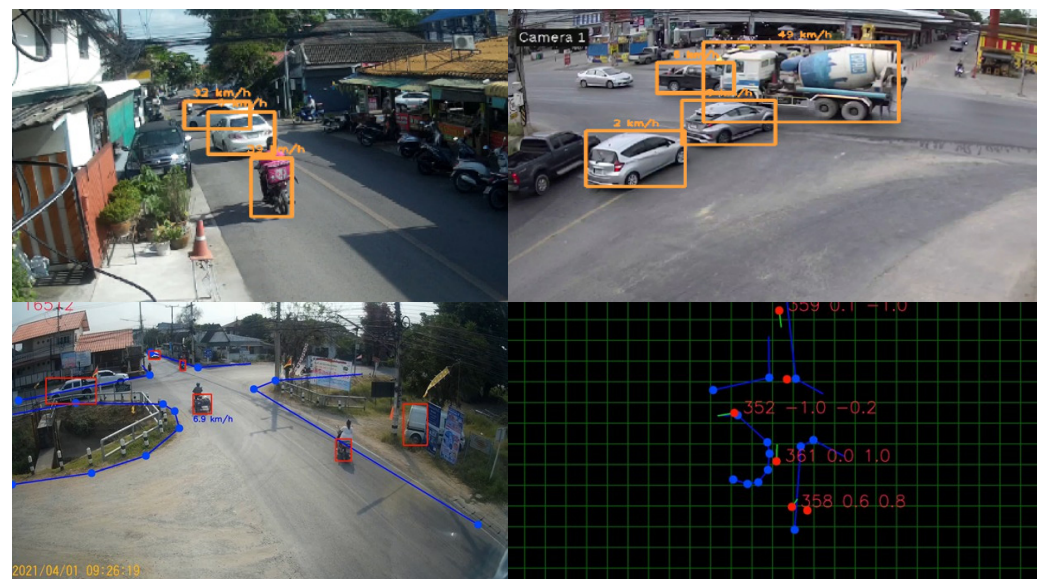
Figure 7. Vehicle detection, classification, and tracking systems in this study.
