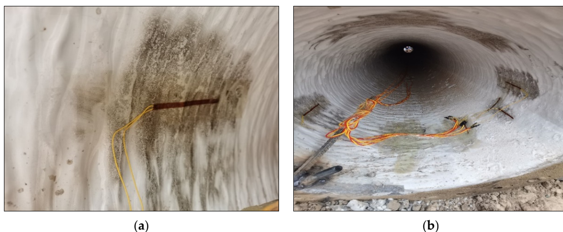
Figure 6. Arrangement of the strain measurement points. (a) Single strain gauge. (b) Strain gauge connection.
