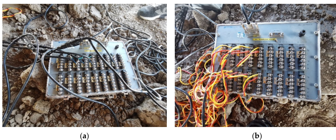
Figure 7. Connection mode of measurement points. (a) Connection mode of displacement measurement points. (b) Connection mode of strain measurement points.
