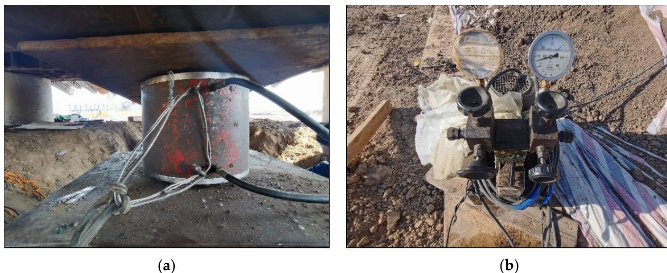
Figure 4. Loading jack. (a) Hydraulic jack. (b) Pressure gauge.
