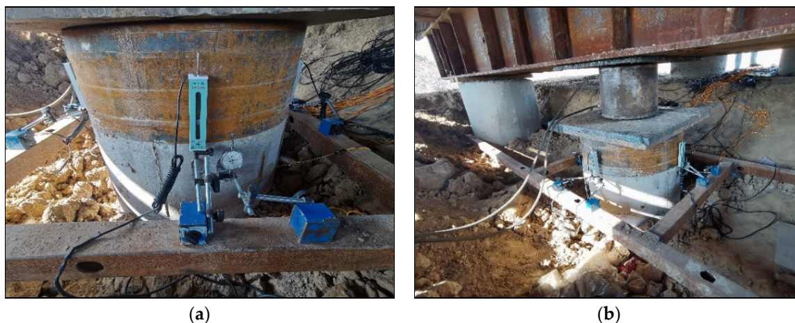
Figure 5. Arrangement of the displacement measurement points. (a) Displacement meters and dial indicators. (b) Reference beam.
