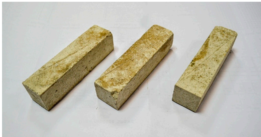
Figure 5. Photo of samples of geopolymer fine-grained concrete.
