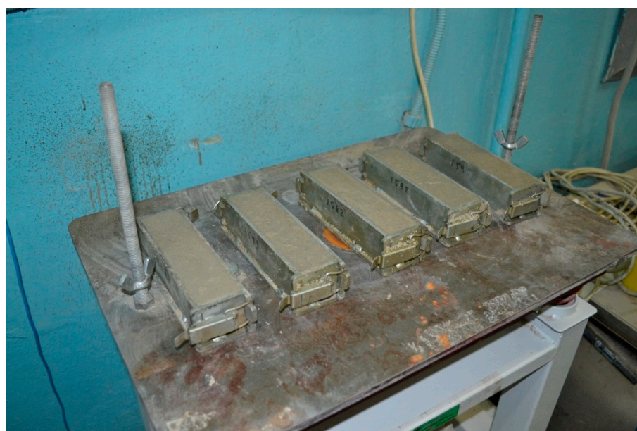
Figure 6. The process of making samples-beams of geopolymer fine-grained concrete.
