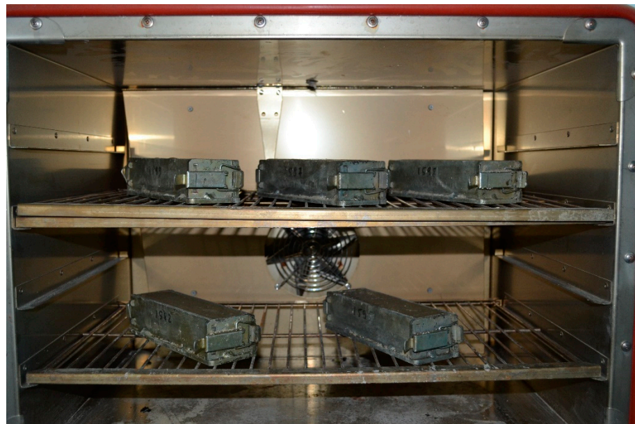
Figure 14. The process of heat treatment of samples—beams of geopolymer fine-grained concrete.
