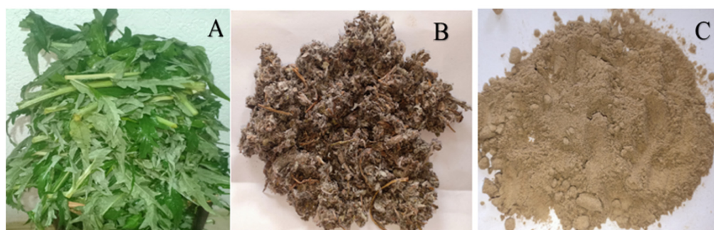
Figure 1. Cardoon waste states: (A) Fresh, (B) Dried, (C) Screened.
