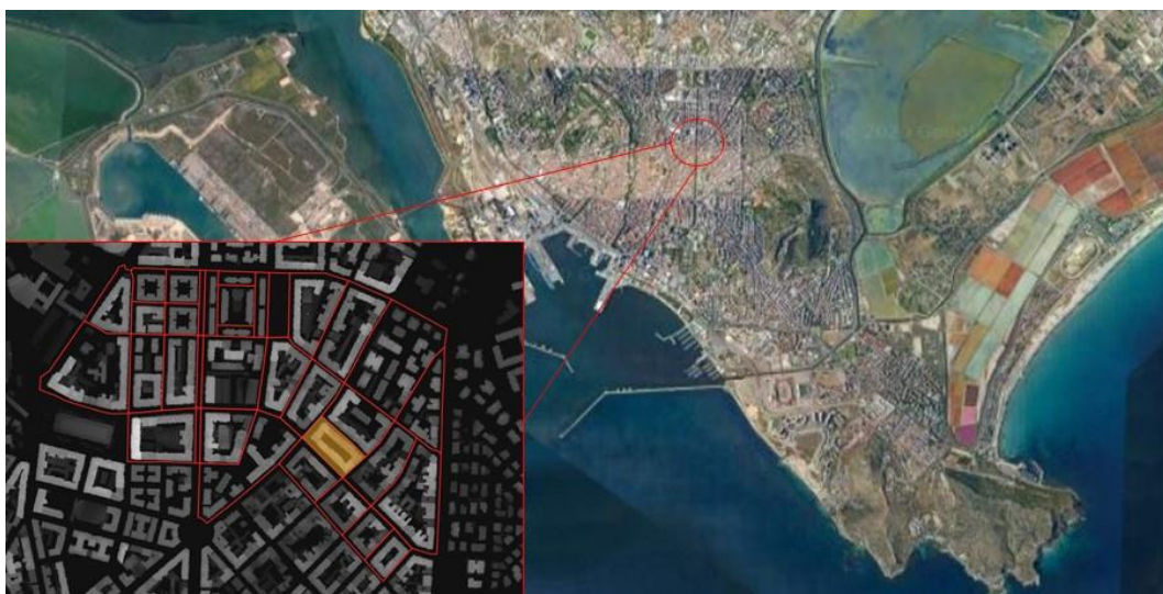
Figure 4. Urban texture sample of Cagliari city. Both raster data and vector data are included, as described in the text. Greyscale represents height values, street graph is reported in red. The example block is highlighted in orange.
