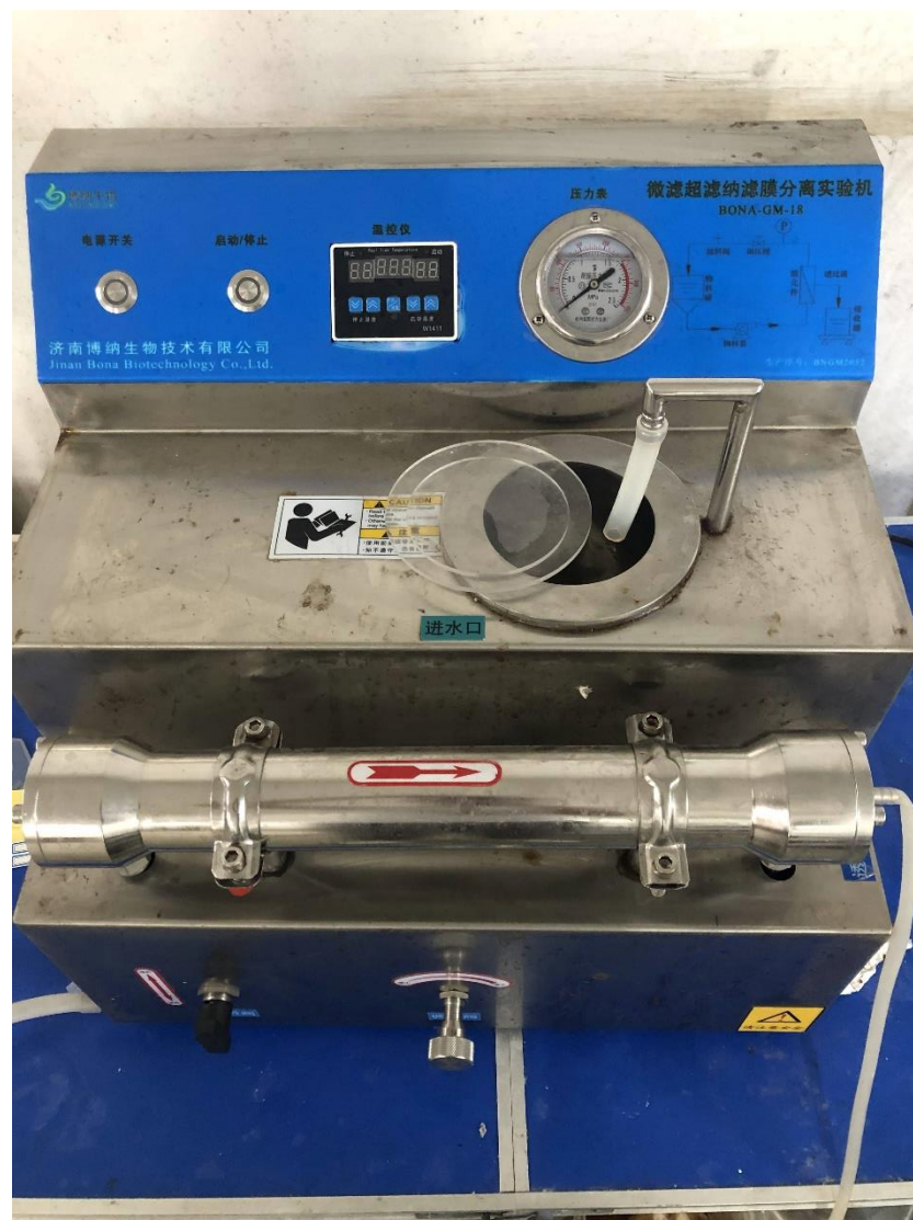
Figure 1. Microfiltration + ultrafiltration + nanofiltration membrane separation experiment machine.
