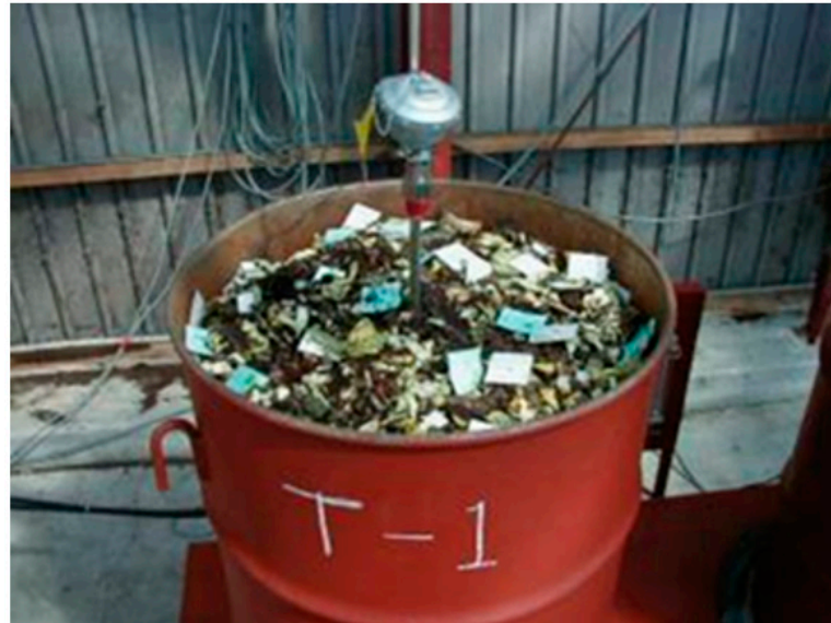
Figure 5. PLA test sample in the pilot-scale compost apparatus.
