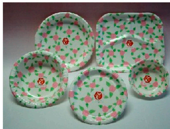
Figure 1. PLA film-laminated paper plates as a test sample.
