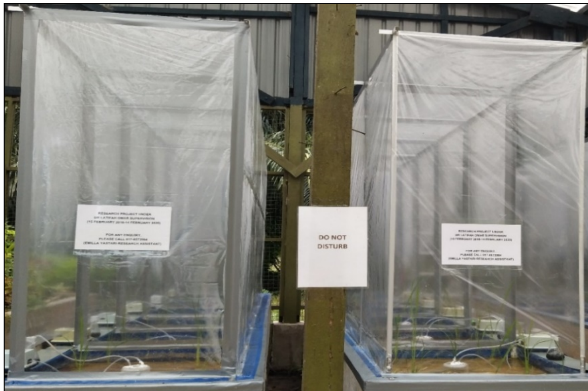
Figure 1. Troughs covered with chambers to accommodate ammonia released which was trapped with boric acid to estimate daily ammonia volatilized.
