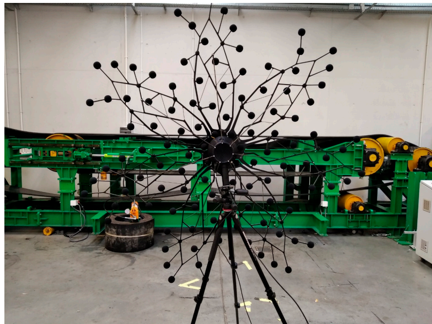
Figure 2. The measurement rig and the location of the Bionic L-112 acoustic camera with respect to the measurement rig.
