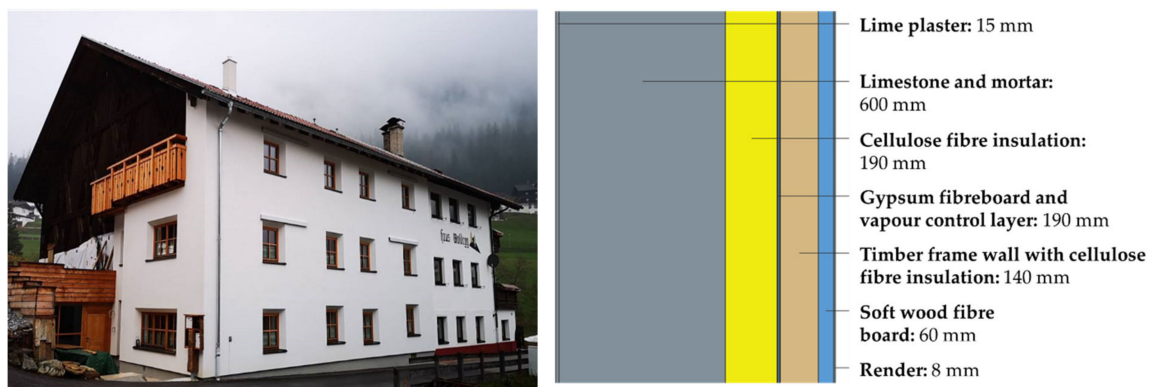
Figure 1. Example of reversible external wall insulation: picture (left) and cross-section ((right), layers presented from inside to outside) [69].
