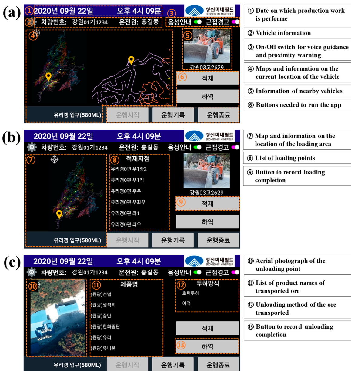
Figure 7. User interface of mine production management app according to the location where the Bluetooth beacon is installed. (a) receiving a signal from a normal beacon on the transport route; (b) receiving a beacon signal attached to a loader located at the loading zone; (c) receiving signals from beacons installed at dumping area.
