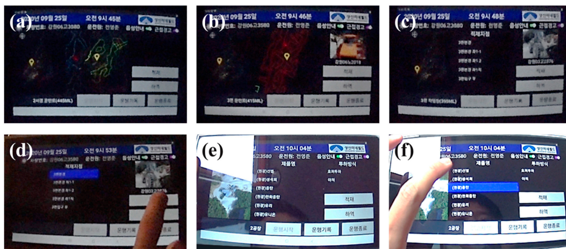
Figure 8. Results of performance experiments. (a) maps and information about the vehicle location; (b) equipment proximity warning; (c,d) loading point selection and input screen; (e,f) product name and dumping method selection and input screen.
