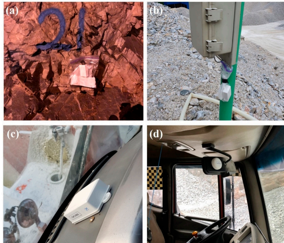
Figure 5. Example of Bluetooth beacon (Beacon i3 and RECO beacon) installed for mine production management app: (a) tunnel wall on the transport route; (b) near the crusher at the crusher 4; (c) dashboard in the driver's seat of the loader; (d) rearview mirror in the driver's seat of the truck.
