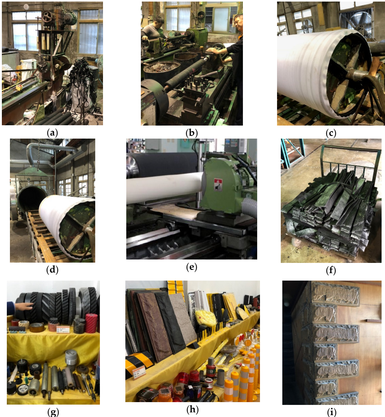
Figure 1. The typical operations for the production in the rubber manufacturer and exemplar rubber products. (a) Compounding; (b) Coating; (c) Molding; (d) Vulcanization; (e) Demolding; (f) Deflashing; (g) Exemplar products of the first line; (h) Exemplar circular products of the second line; (i) Stone-like wall rubber.
