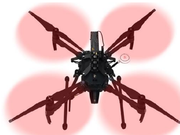
Figure A2. Integration of Sniffer4D unit with DJI M100 quadcopter [39].
