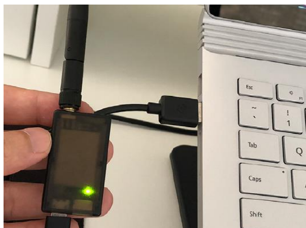
Figure A5. Telemetry module connected to the computer [39].
