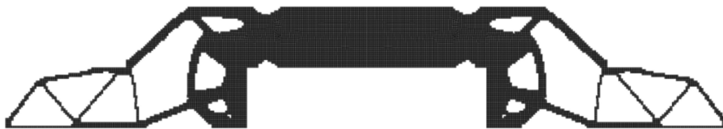
Figure 4. The final topology of the considered structure under mass constraint.
