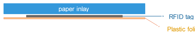
Figure 8. Structural scheme of the RFID tag No. 4 placed between a textile inlay and a plastic foil.
