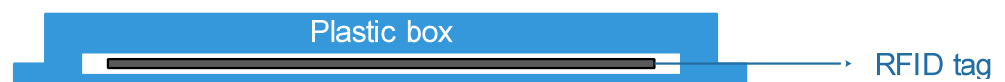
Figure 3. Structural scheme of the RFID tag No. 2 placed in a plastic box.
