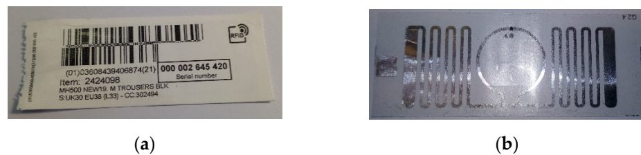
Figure 7. RFID tag No. 3: (a) general view; (b) partially extracted RFID tag.
