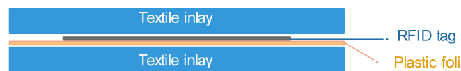
Figure 6. Structural scheme of the RFID tag No. 3 placed between textile inlays on a plastic foil.
