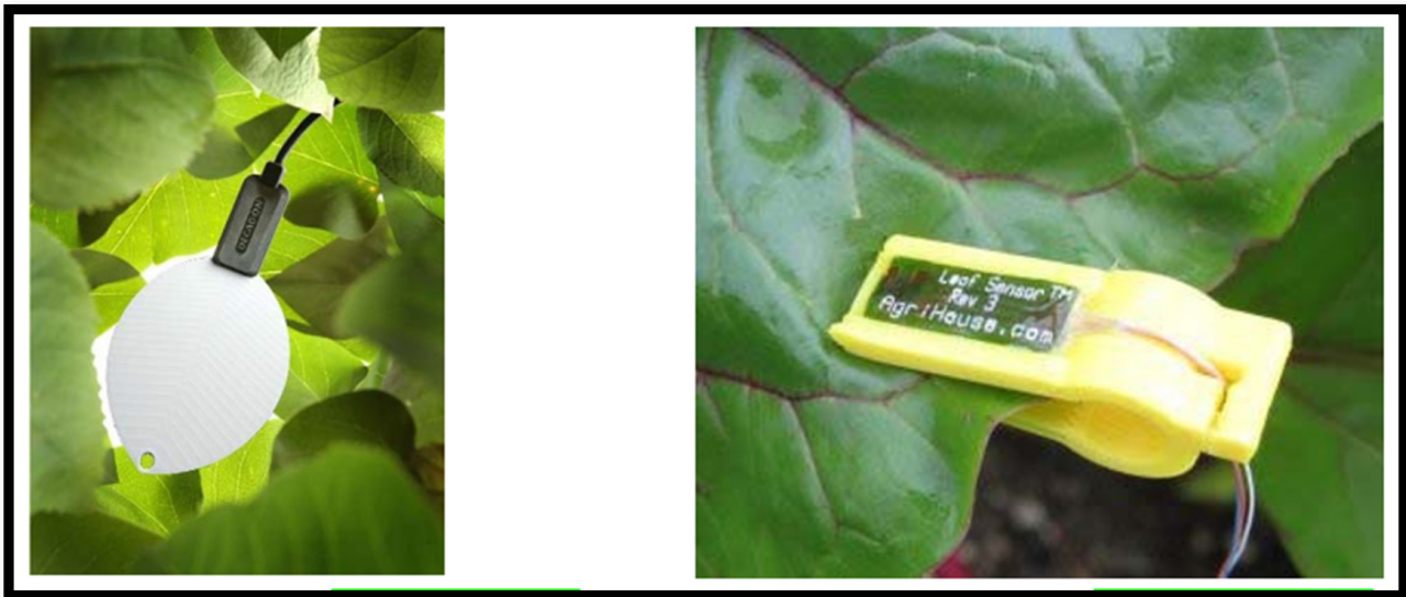
Figure 5. Decagon leaf wetness sensor (left image) and AgriHouse leaf sensor (right image) [41].
