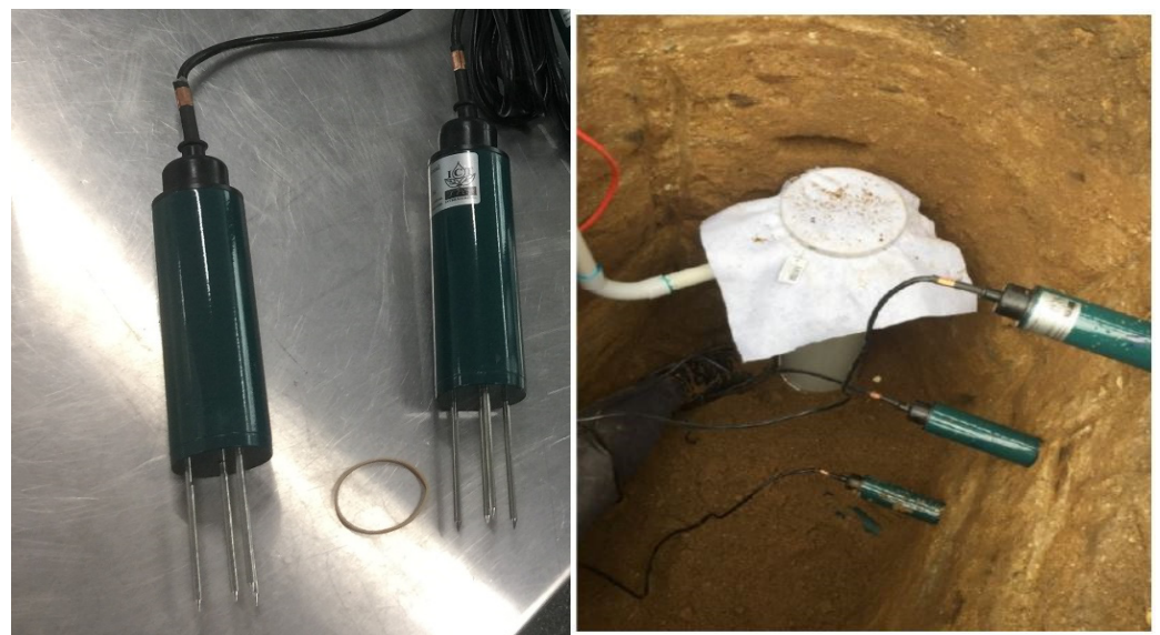
Figure 4. MP406 soil moisture sensor (left image) and sensors implanted in different depth of soil (right image) [37].
