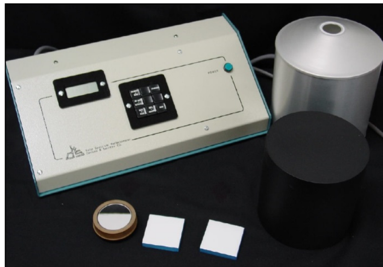
Figure 3. Solar spectrum reflectometer.
