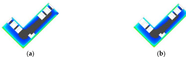
Figure 16. Overall Achieved Day Light Levels (110 lux to 2200 lux) on (a) 2nd Floor (b) 3rd Floor.
