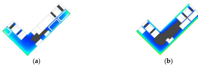
Figure 15. Overall Achieved Day Light Levels (110 lux to 2200 lux) on (a) Ground Floor (b) 1st Floor.
