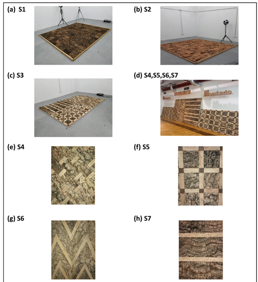
Figure 2. Samples tested in the reverberation chamber: (a) S1; (b) S2; (c) S3; (d) S4, S5, S6, and S7; and some details of the samples: S4 (e); S5 (f); S6 (g); S7 (h).
