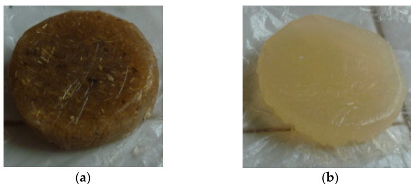
Figure 2. Composite structures based on starch: (a) rapeseed residues with starch; (b) gelled starch.
