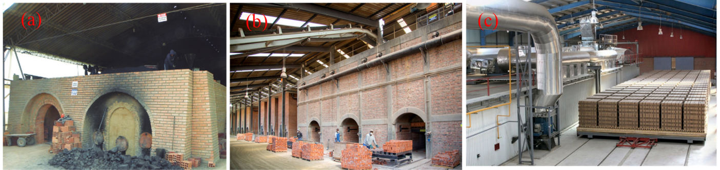
Figure 2. Relative high-tech brick kilns: (a) zig-zag kiln; (b) Vertical shaft brick kiln; and (c) Tunnel kiln.
