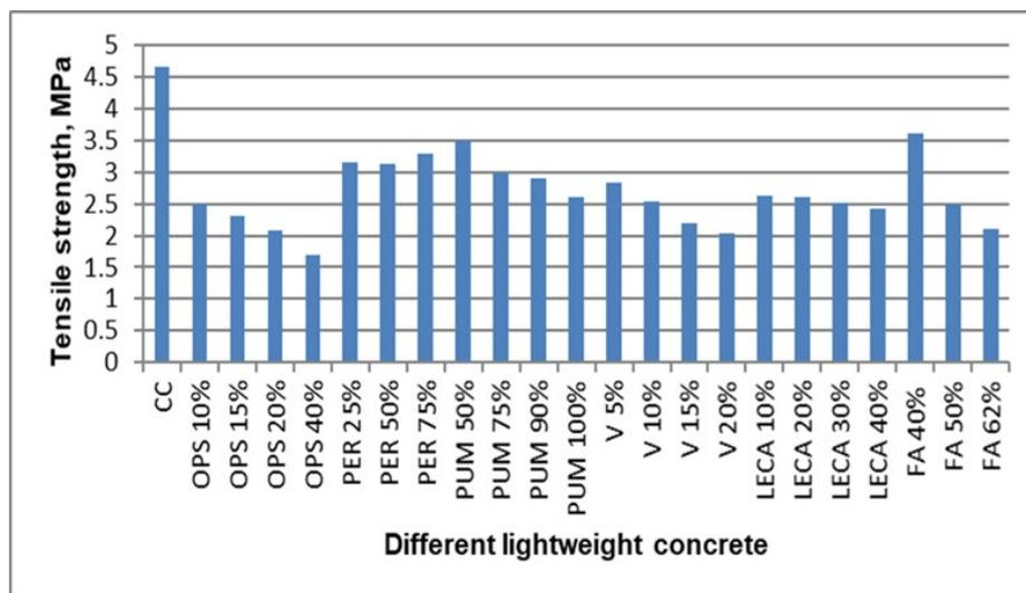
Figure 13. Tensile strength of different LWACs.
