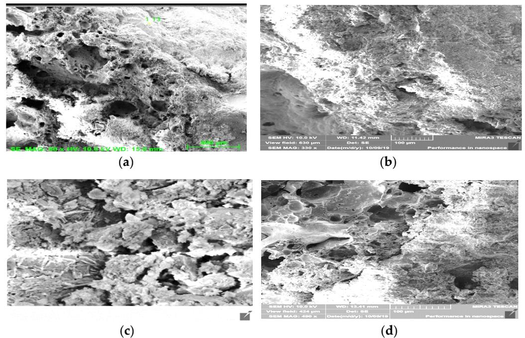
**Figure 17.** SEM Results of laboratory prepared LWAC specimens. (a) Control concrete; (b) FA 30%; (c) MS 30%; (d) FA15% + MS15%.
