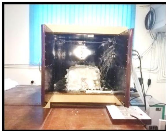
**Figure 16.** Thermal conductivity test set up for LWAC containing fly ash and marble waste.
