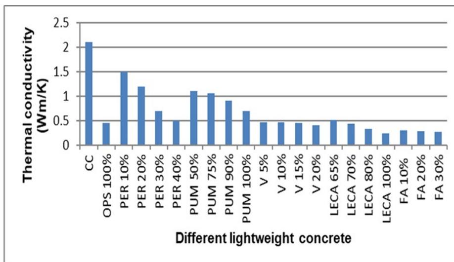
Figure 15. Thermal conductivity of different LWACs.
