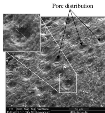
**Figure 5.** Micro-pores on outer surface [54]. (Reprinted with permission from Alengaram et al. (2011), 2021, Elsevier).
