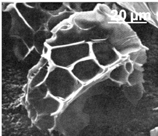
**Figure 8.** SEM micrographs of perlite [42]. (Reprinted with permission from Abidi et al. (2015), 2021, Elsevier).
