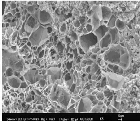
**Figure 9.** The pore structure of the perlite in the fly ash–lime–gypsum mixture [72]. (Reprinted with permission from Demir and Baspinar (2008), 2021, Elsevier).
