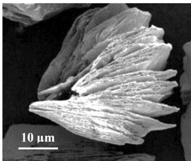
**Figure 7.** SEM micrograph of vermiculite [42]. (Reprinted with permission from Abidi et al. (2015), 2021, Elsevier).
