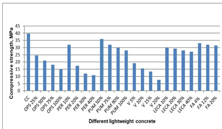
**Figure 12.** Compressive strength of different LWACs.
