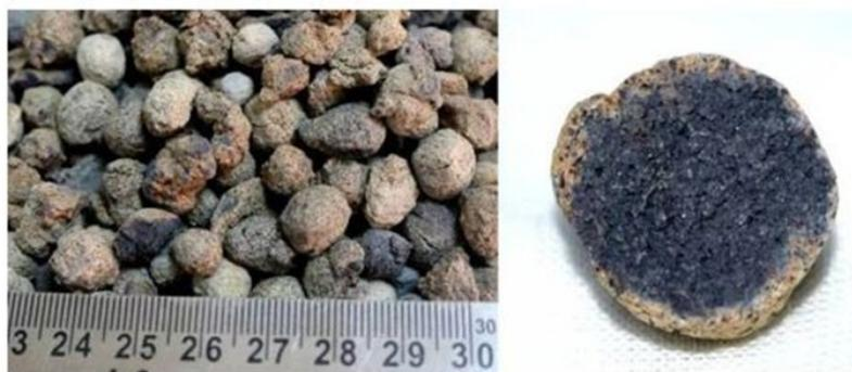
**Figure 10.** Sintered FA aggregates (left) and their cross-section (right) [76]. (Reprinted with permission from Nadesan and Dinakar (2017), 2021, Elsevier).
