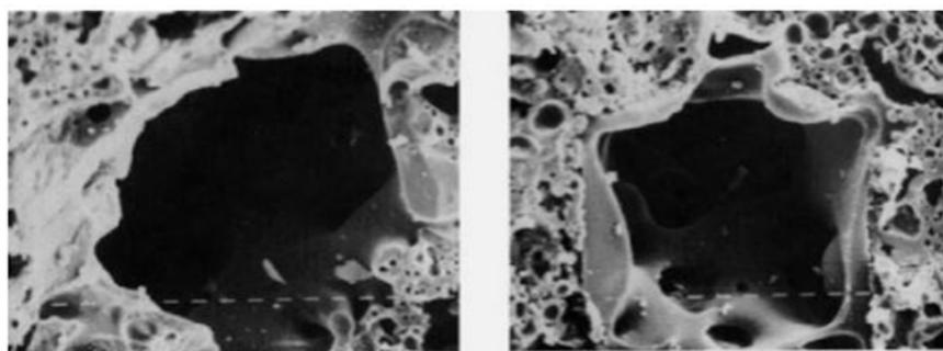
**Figure 11.** Microstructure of sintered fly ash aggregate ( $\times 320$ ) [77]. (Reprinted with permission from Swamy and Lambert (1981), 2021, Elsevier).
