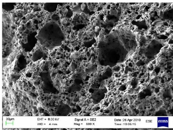
**Figure 6.** Surface image of a LECA particle under SEM showing pores [56]. (Reprinted with permission from Nkansah et al. (2012), 2021, Elsevier).
