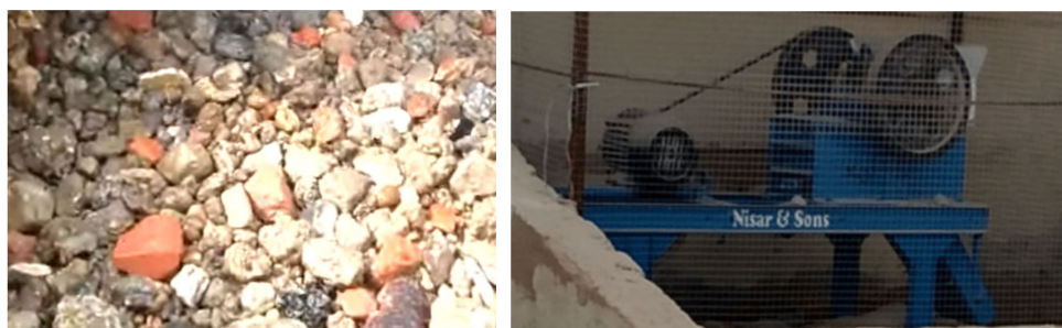
Figure 1. Crushed RCA (on left) and Jaw Crusher (on right).
