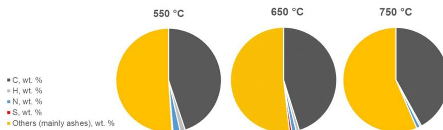
**Figure 5.** Compositional analysis of char samples derived from RDF fast pyrolysis tests at 550 °C, 650 °C, and 750 °C. C, H, and N contents were determined in accordance with the ASTM D3176 protocol by using a Leco 628 elemental analyser. S content was measured in accordance with the ASTM D4239 protocol by using a Leco 144 analyzer.
