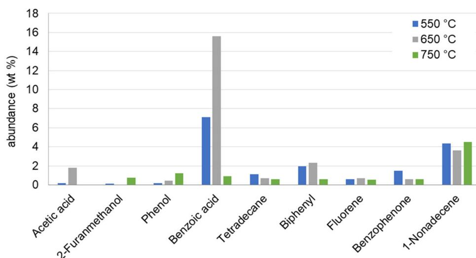
**Figure 4.** Relative abundance of selected species in bio-oils from RDF fast pyrolysis tests at 550 °C, 650 °C, and 750 °C. The abundances have been estimated by gas chromatographic analysis of acetone-diluted bio-oil solutions performed on an Agilent GC-MS instrument (7890 A/5972 C) equipped with an Agilent DB-624 capillary column.
