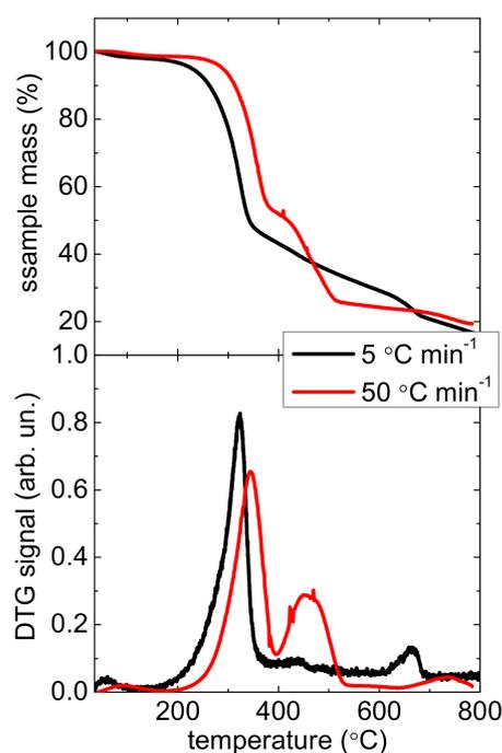
**Figure 3.** Mass loss (upper panel) and corresponding derivative curve of a RDF. Thermogravimetric analyses have been performed from 30 °C up to 800 °C on a Perkin–Elmer STA6000 under inert atmosphere (N<sub>2</sub>, flux 40 mL/min), applying two different heating rates: 5 °C/min and 50 °C/min.
