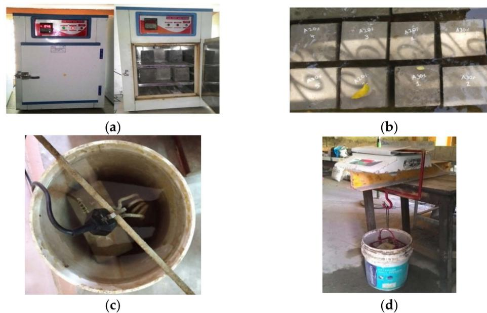
**Figure 4.** (a) Samples in oven drying; (b) samples immersed in water; (c) samples in boiling water; (d) Sample in apparent basket.
