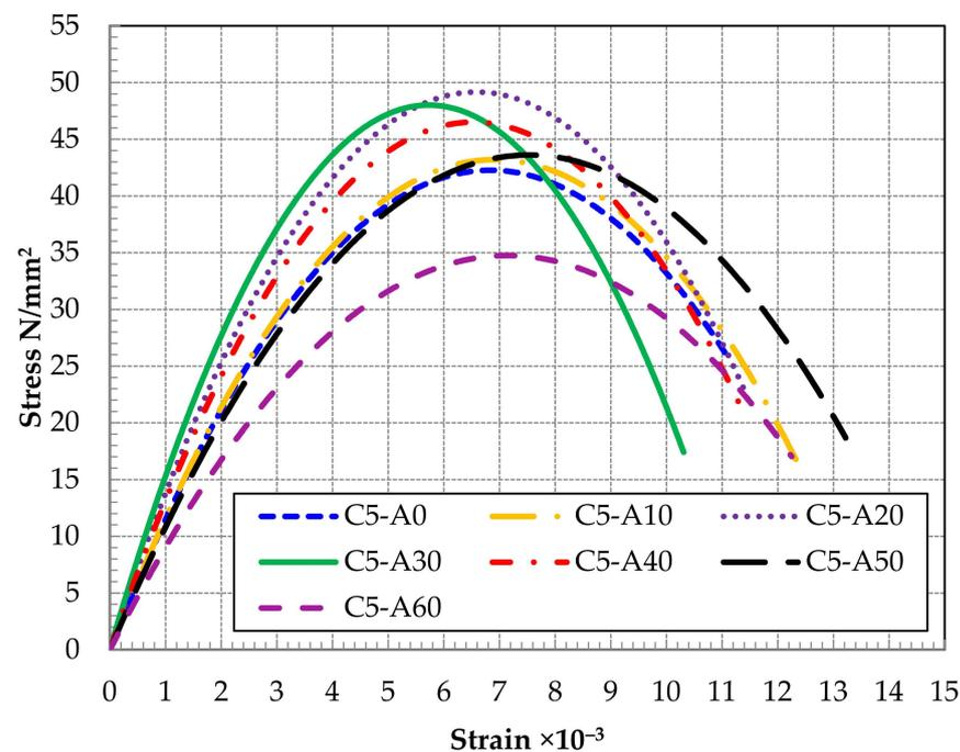
**Figure 11.** Stress–strain curves of SCC mixes with varying % of alccofine.
