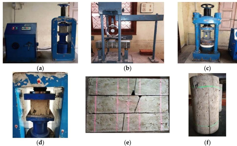
**Figure 3.** Testing of specimens in laboratory (a–c). Test setup of compression, flexure, and E-for concrete and (d–f) failure pattern of cube, prism, and cylinder.
