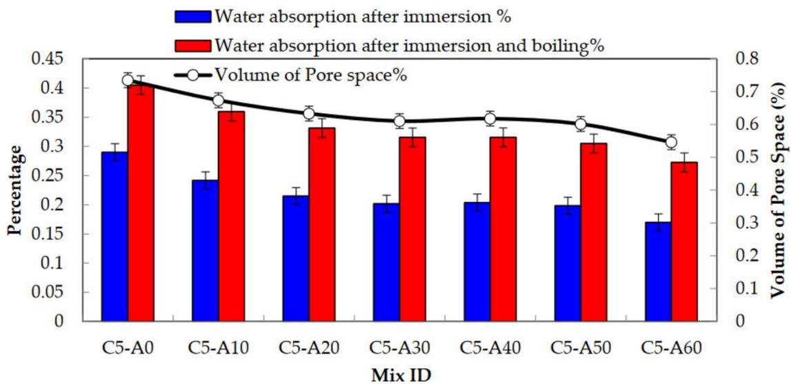
Figure 15. Water absorption and pore space percentage of SCC mixes.
