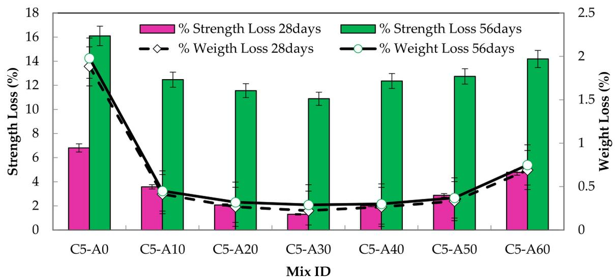
Figure 18. Percentage of strength and weight loss due to sulphate attack.
