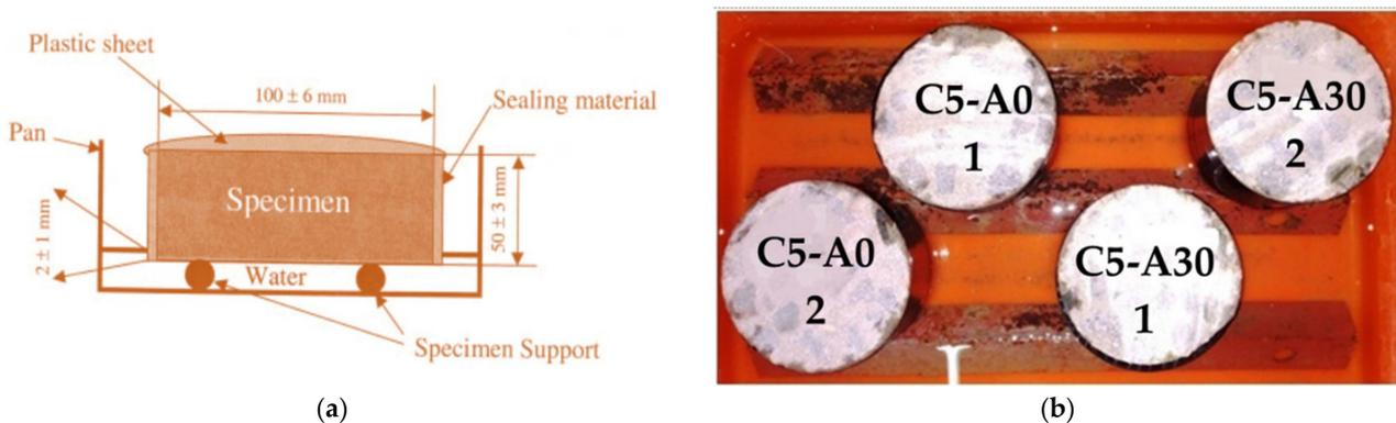
**Figure 5.** (a) Schematic procedure of sorptivity and (b) samples placed in the sorptivity pan.
