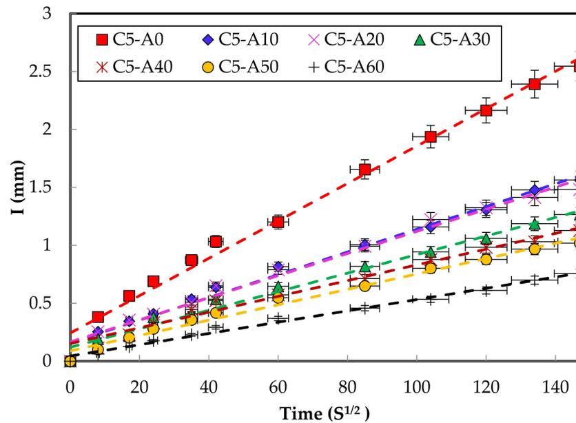
Figure 17. Initial rate of absorption of SCC mixes.
