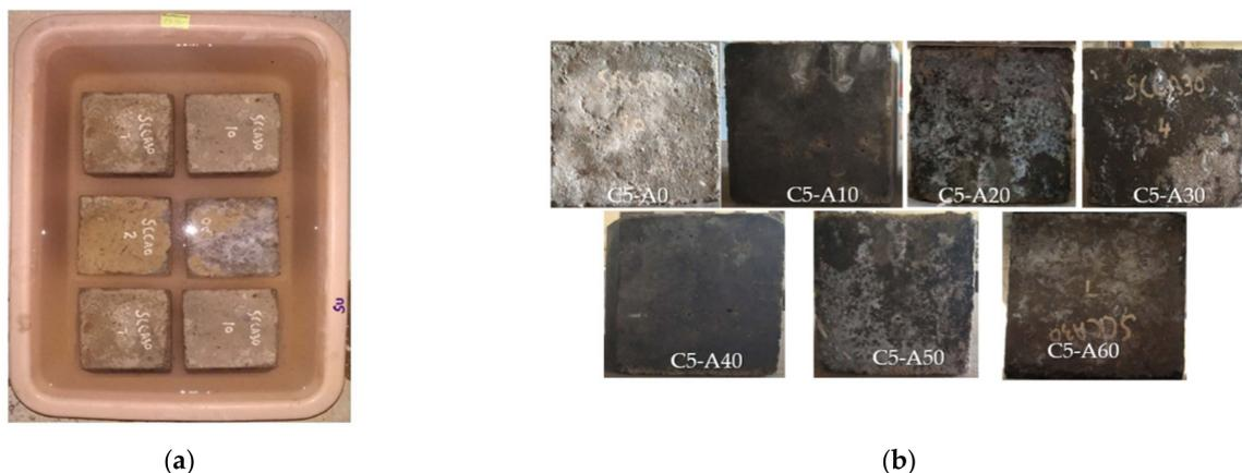
**Figure 6.** (a) Specimens immersed in  $MgSO_4$  solution and (b) specimens after immersion in  $MgSO_4$  solution.
