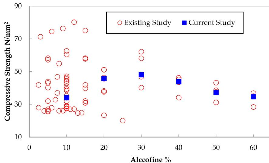
**Figure 12.** Comparison of compressive strength with existing findings.
