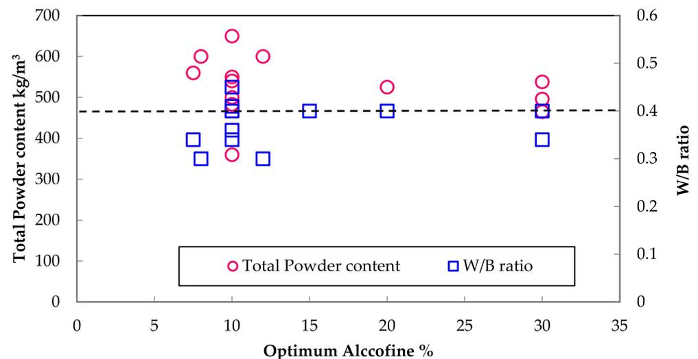
Figure 14. Interpretation between the optimum percentage of alccofine with total powder content and the W/B ratio.
