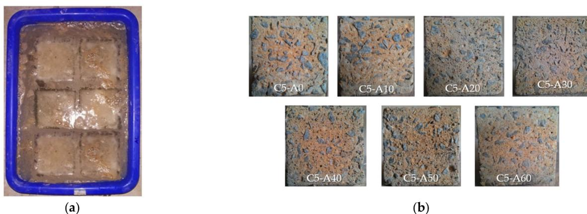
**Figure 7.** (a) Specimens immersed in HCl solution and (b) specimens after immersion in HCl solution.
