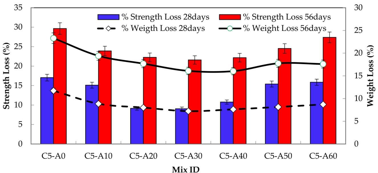
**Figure 19.** Percentage of strength and weight loss due to acid attack.
