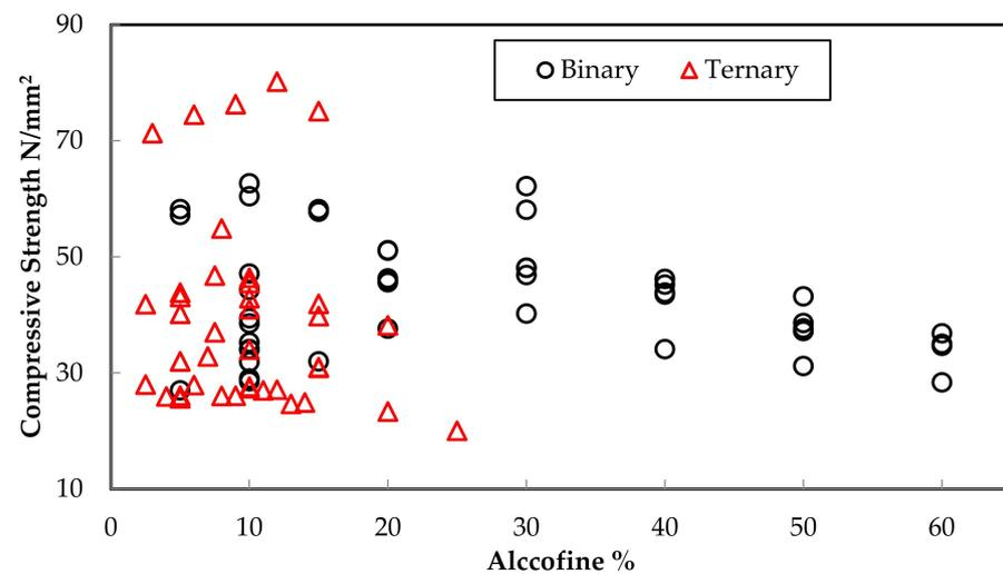
Figure 13. Comparison of compressive strength as binary and ternary combination with existing findings.
