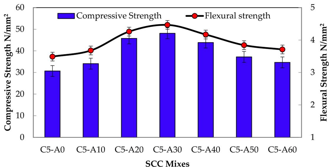
**Figure 10.** Compressive and flexural strength of SCC mixtures.
