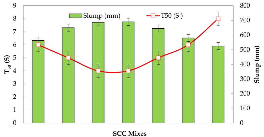
**Figure 8.** Slump flow and T<sub>50</sub> time of SCC mixtures.
