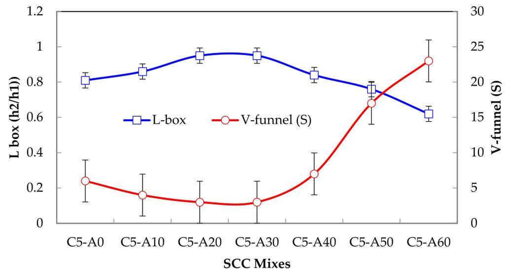
**Figure 9.** V-funnel time and L-box ratio of SCC mixtures.
