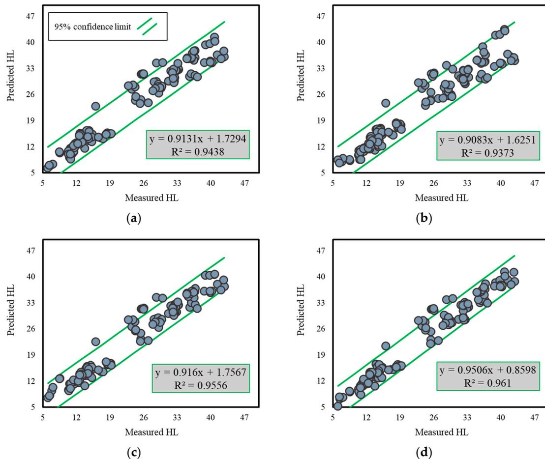
**Figure 7.** Measured testing CLs vs. prediction of (a) FA-MLP, (b) OIO-MLP, (c) SCE-MLP, and (d) TLBO-MLP.
