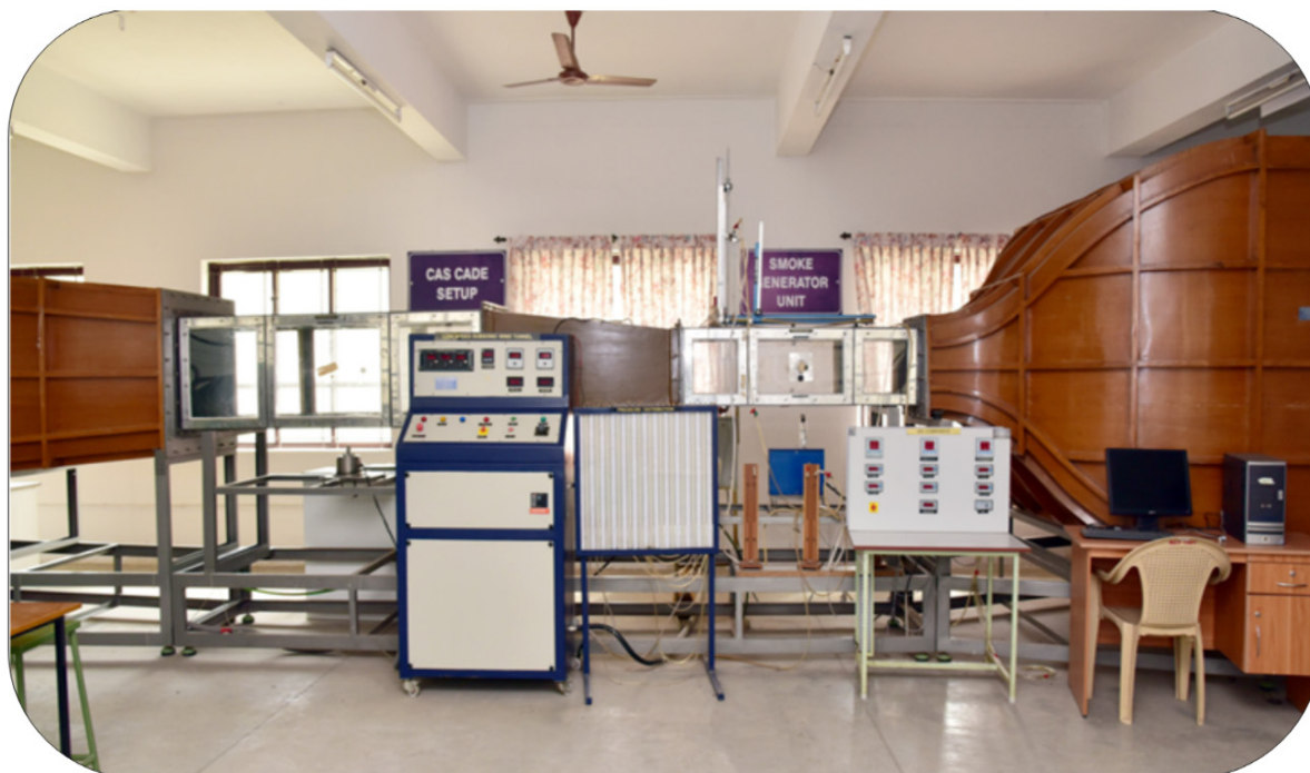
Figure 20. Typical full view of the subsonic wind tunnel with the data acquisition system (bottom right).
