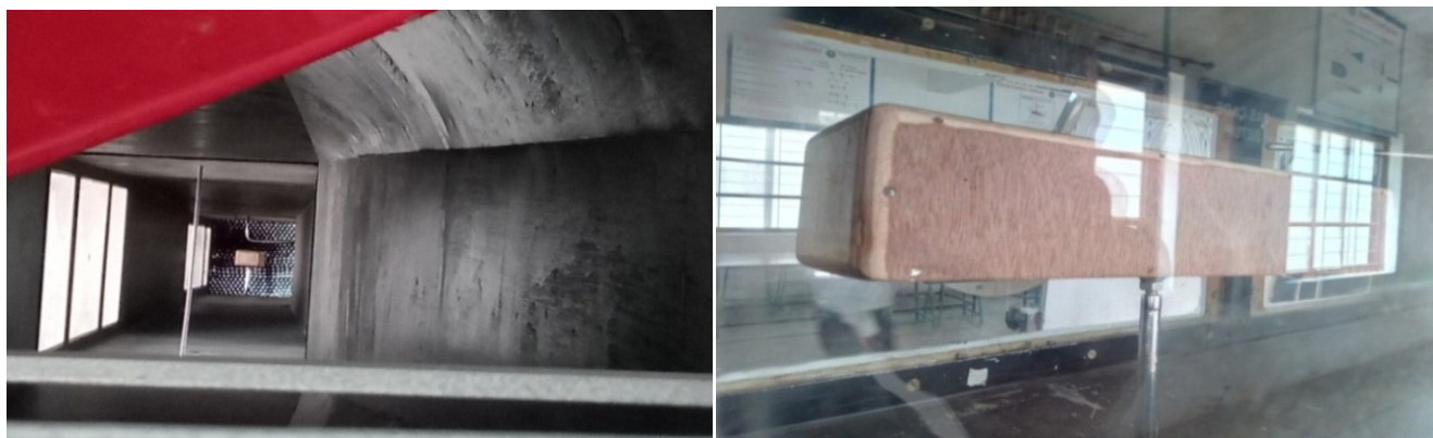
Figure 21. Typical zoomed-in and normal views of an intercity bus without dimples located in the test section.
