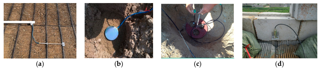
Figure 5. Monitoring instruments: (a) strain gauge; (b) earth pressure cell; (c) settlement meter; (d) displacement meter.
