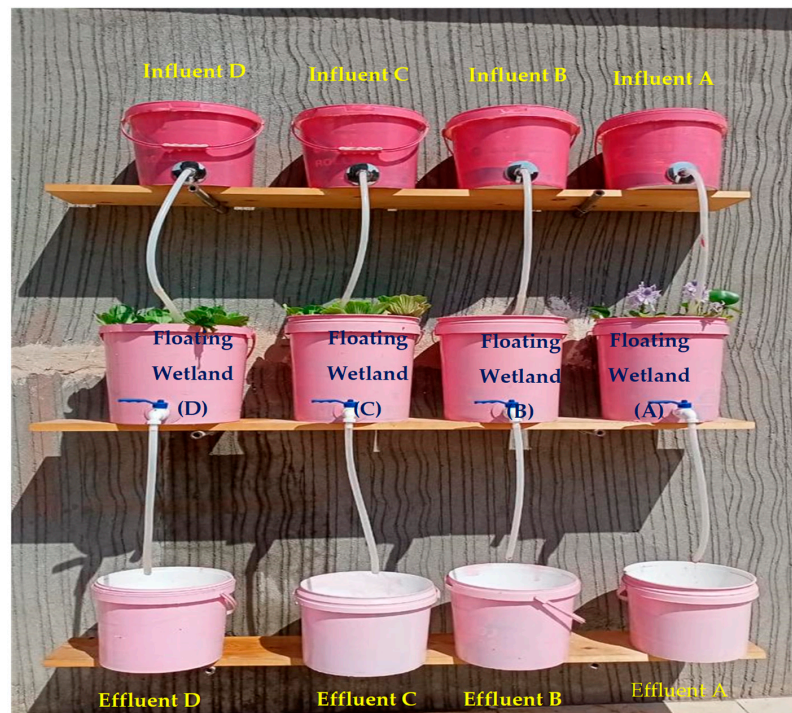
Figure 2. Experimental floating wetland setup, (A) Eichhornia , (B) Ceratophyllum , (C) Pistia stratiotes , and (D) Nymphaea lotus .
