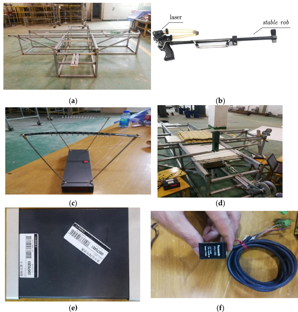
Figure 3. FEM model. (a) Structure of bracket. (b) The details of catapult. (c) The speedometer. (d) The manual windlass. (e) The data acquisition card. Non-English word in the figure mean the care belong to school (f) Laser displacement sensor. Non-English word in figure shows the sensor type.
