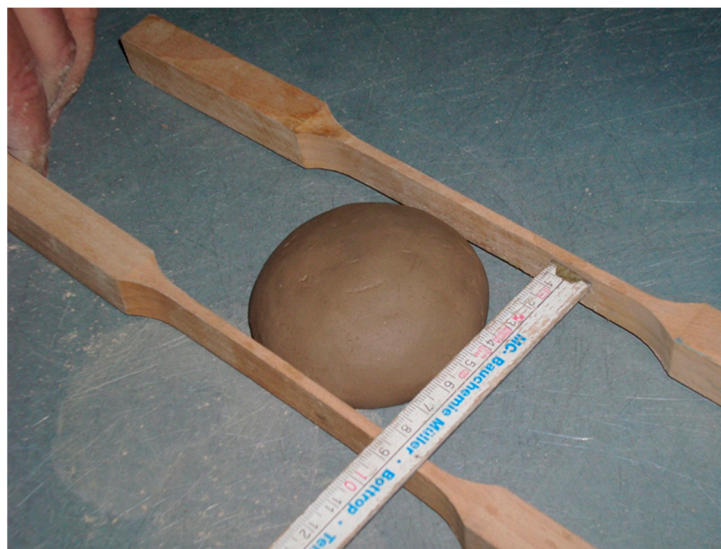
Figure 2. 200 g clay ball after falling from the height of 2 m.
