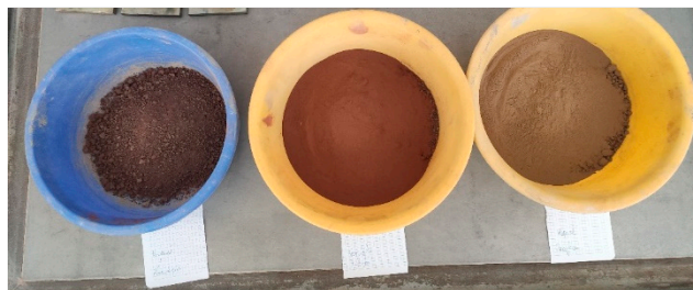
Figure 1. Fly ash from thermal conversion of sewage sludge obtained in three sewage treatment plants.
