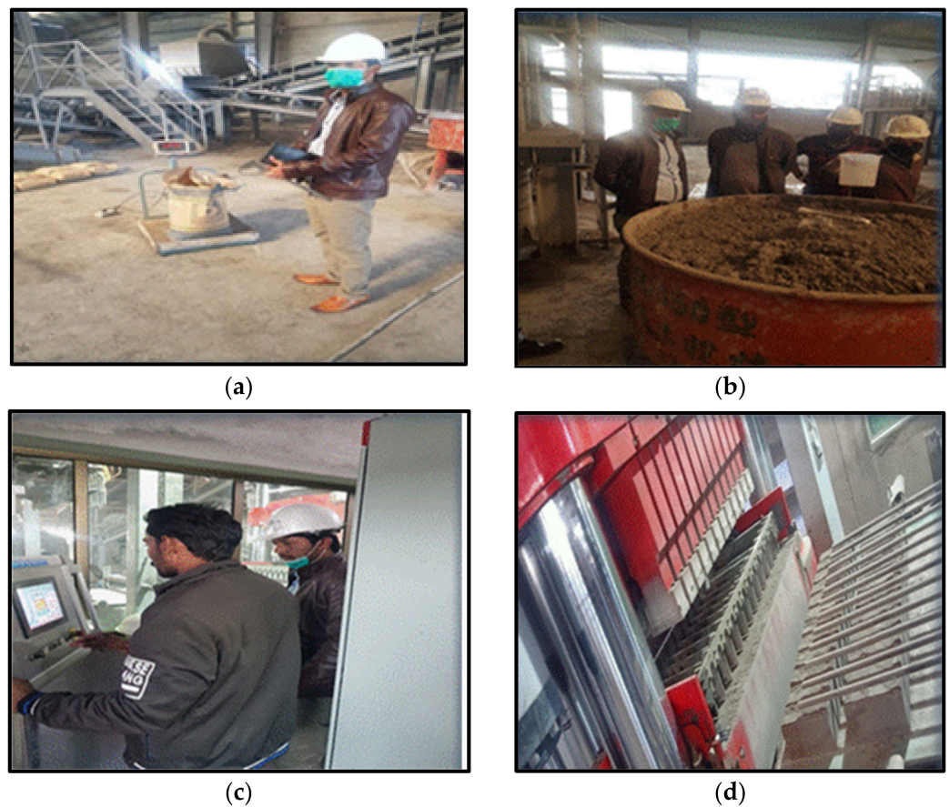
Figure 1. Different stages in the preparation of CA bricks i.e., (a) weighing (by weight) of mixed materials, (b) pan mixing of mixed ingredients, (c) automatic pressure control system, and (d) and application of forming pressure on bricks.
