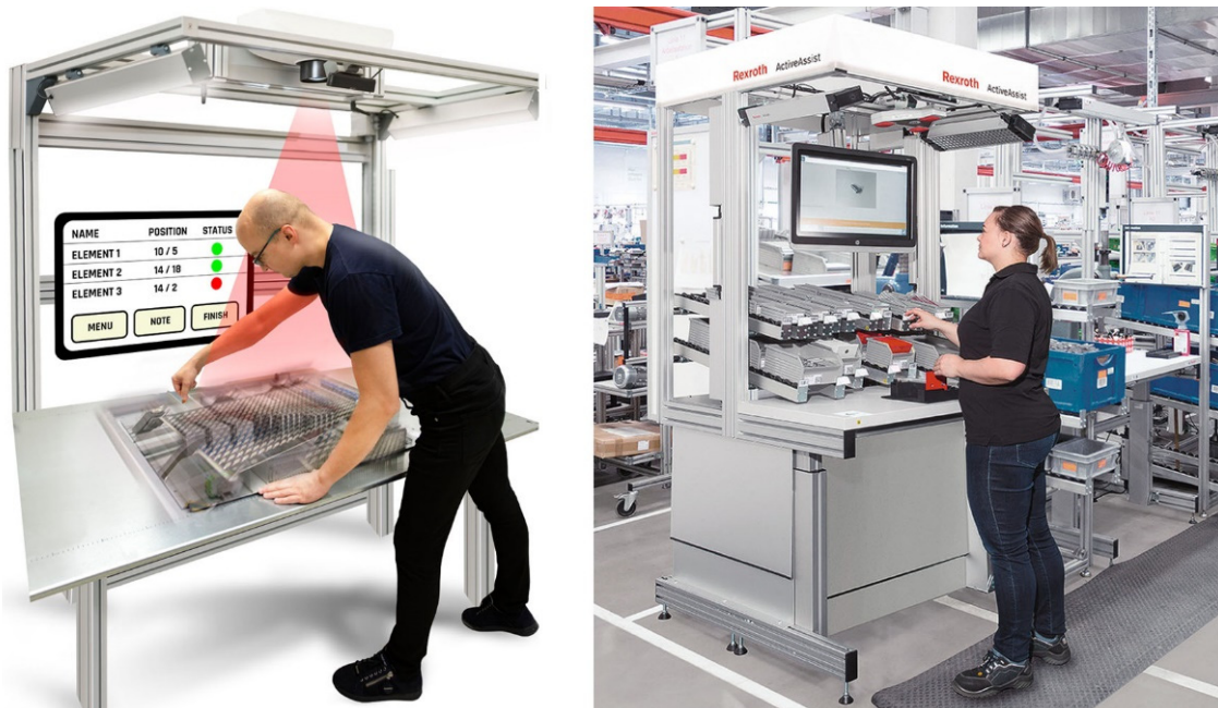
Figure 4. Examples of SAR—stationary AR. Left: DTPoland intelligent station (source: the current authors' workplace); right: Bosch Rexroth ActiveAssist workstation [74].
