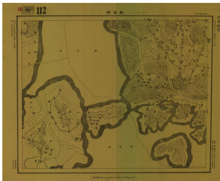
Figure 2. Military topographic map of 1:50,000 in 1930s. This map is a series of topographic maps of the Poyang Lake area in Jiangxi Province. The area shown in the map is the lake surface near Duchang County of Poyang Lake, and the main landform types are lakeside dunes and paddy fields.
