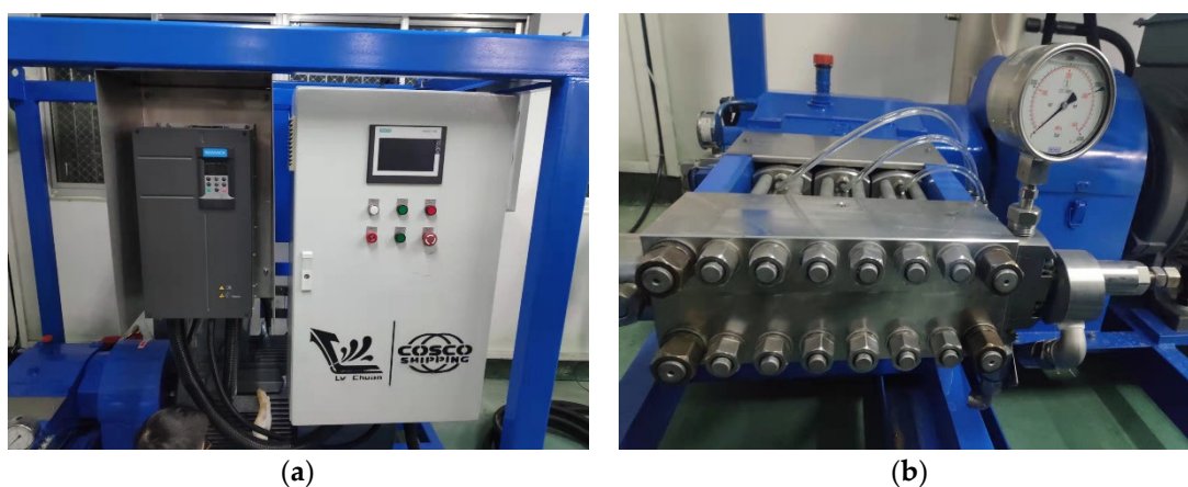
Figure 10. Water jet experimental platform. (a) Control system. (b) ultra-high pressure pump.
