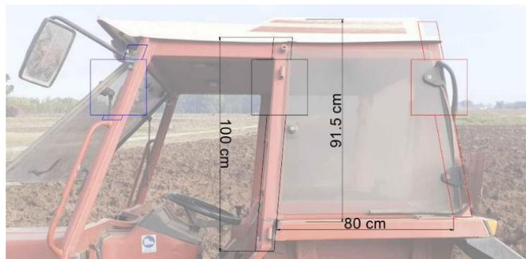
**Figure 4.** Three anchorages for antennas. Blue (front), black (middle) and red (rear).
