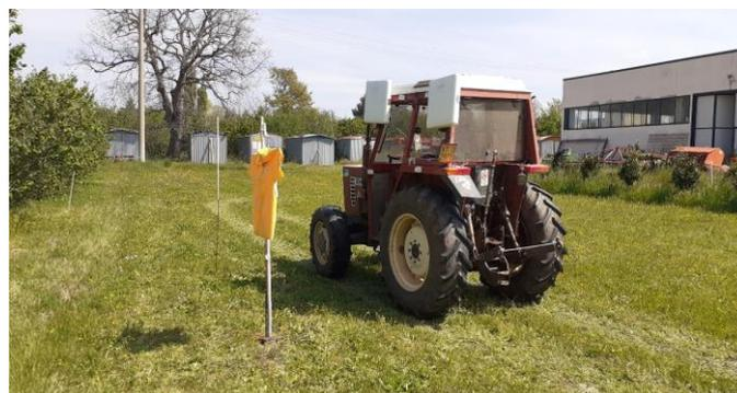
Figure 7. Tractor performing field tests. Antennas are visible on tractor's cab and passive RFIDs have been placed on obstacles and poles all around the area.
