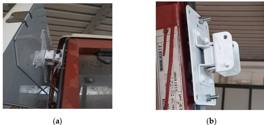
**Figure 5.** Anchorage details: (a) VESA 200 support for the xArray antenna; (b) anchorage bolts already available on tractor's cab, plus pan-tilt plate for further adjustments.
