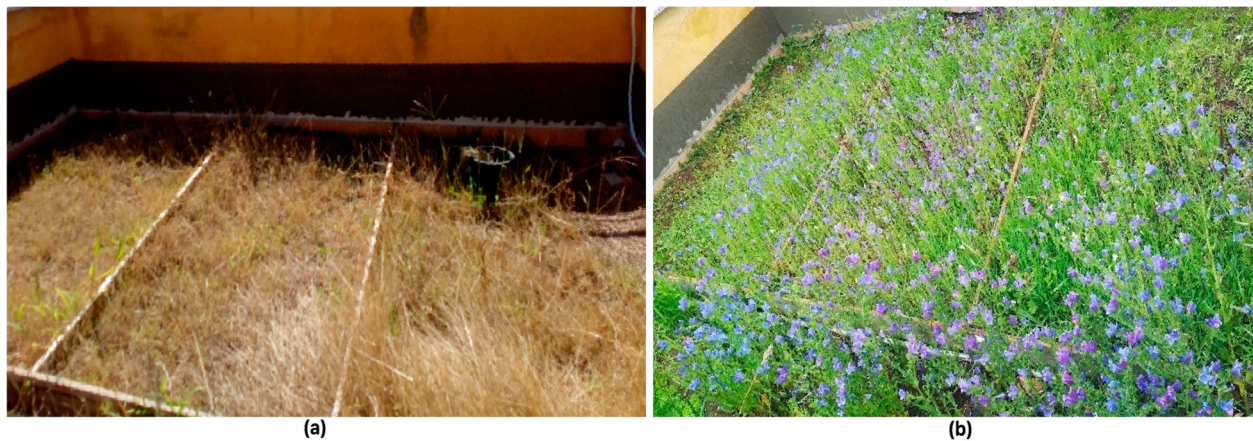
Figure 6. ENEA green roof sector with all vegetation completely dried after water stress imposition at the end of September 2019 (a). Vegetative blooming in April 2020 of Echium plantagineum , showing a high capacity for self-regeneration from the severe dehydration (b).
