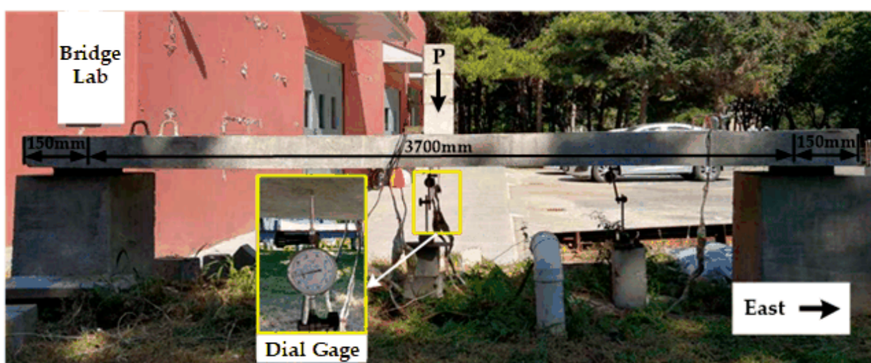
Figure 5. The simply supported bridge.
