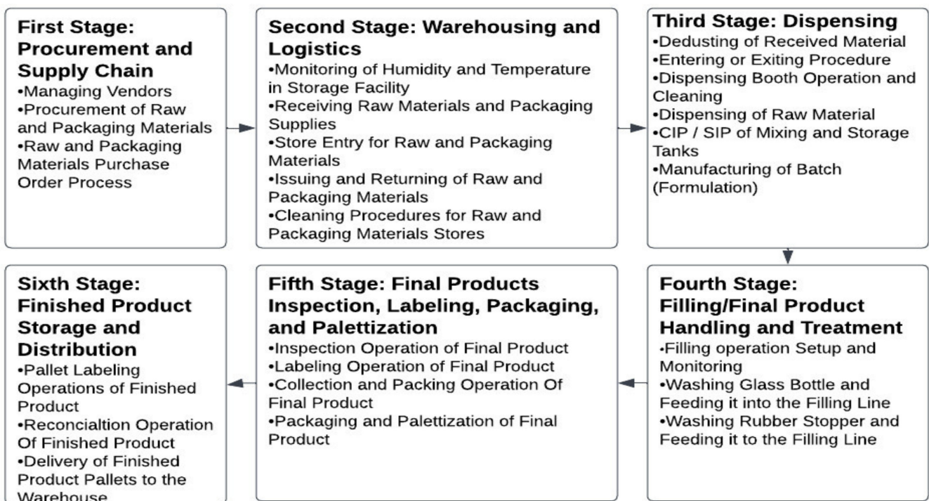
Figure 1. Stages of Manufacturing for a Sterile Drug Product in Glass Bottle (100 mL). Stage four is the focus of this study.
