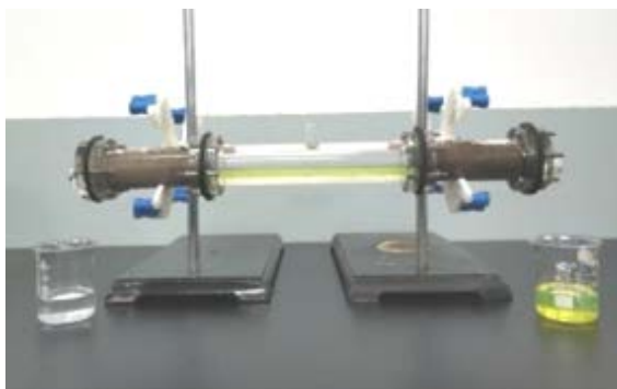
Figure S4. Separation device for oil and water mixture.
