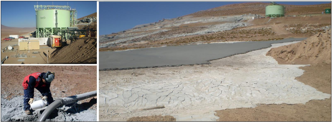
Figure 14. Demo Plant overview and paste tailings disposal at TSF [36,50].
