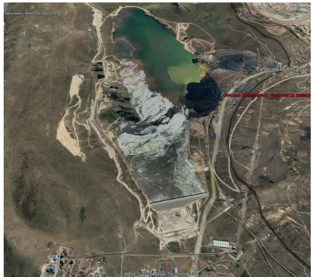
Figure 66. Huachuacaja Thickened TSF Layout.
