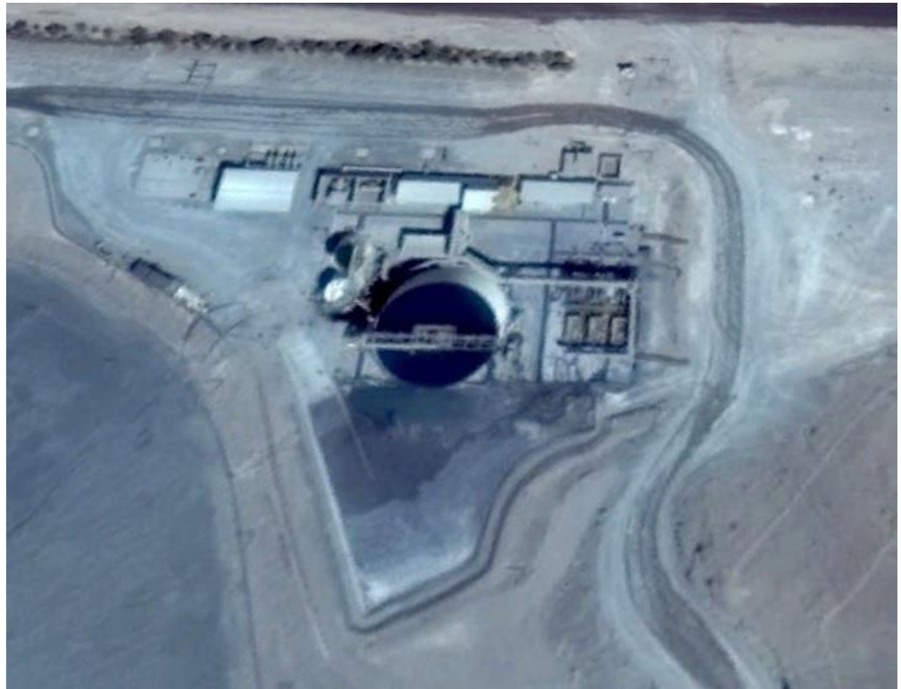
Figure 38. Coemin Tailings Thickening Plant.
