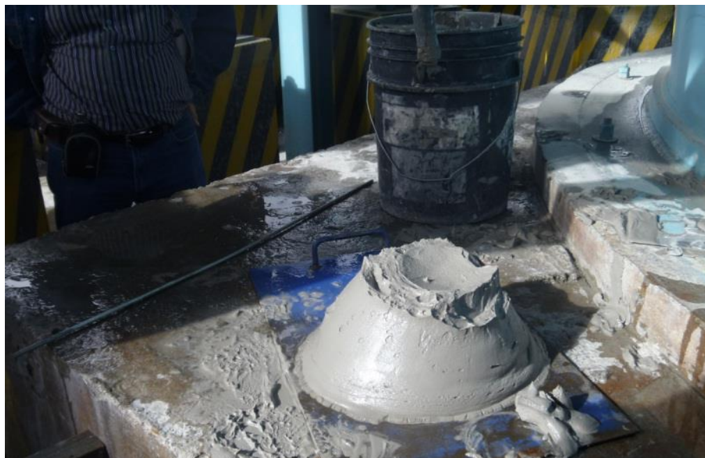
Figure 57. Paste Tailings Viscosity and Consistency—Chungar Thickening Plant.
