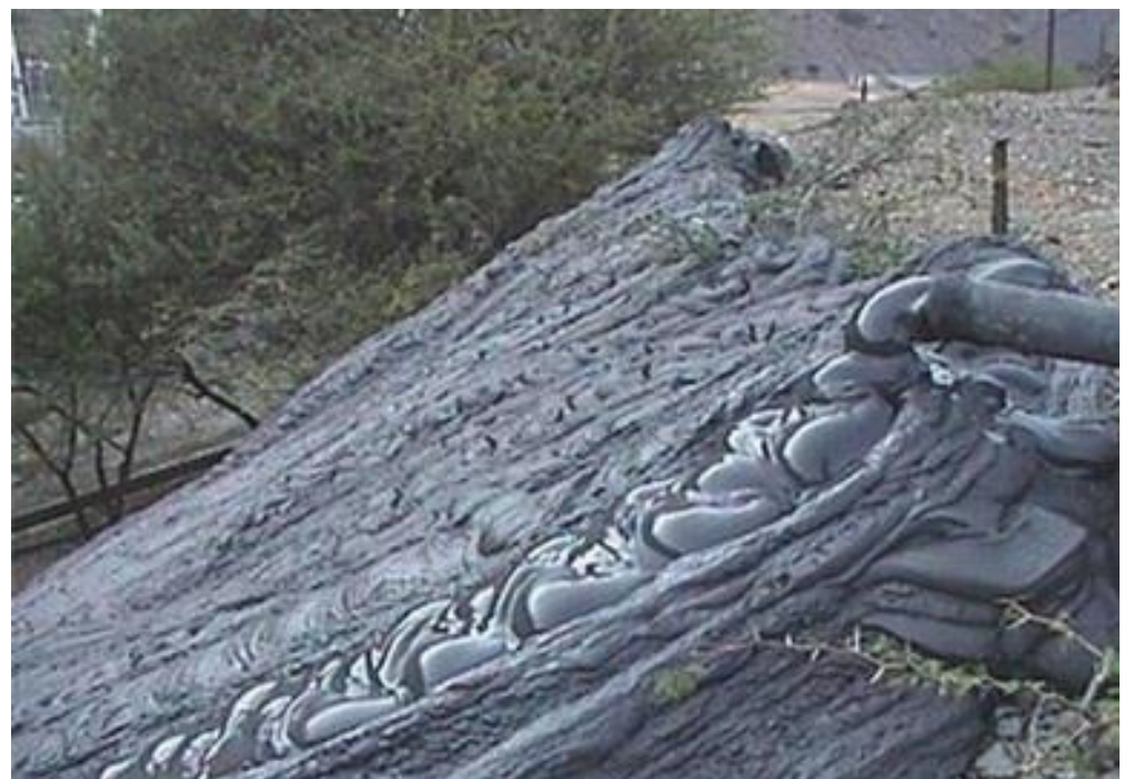
Figure 61. High Viscosity in Cobriza Paste Tailings Disposal.
