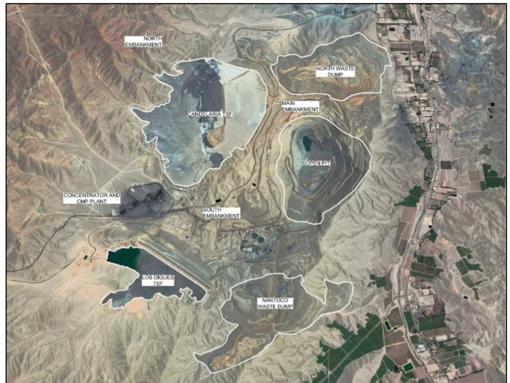
Figure 35. Layout Candelaria Mining Project.
