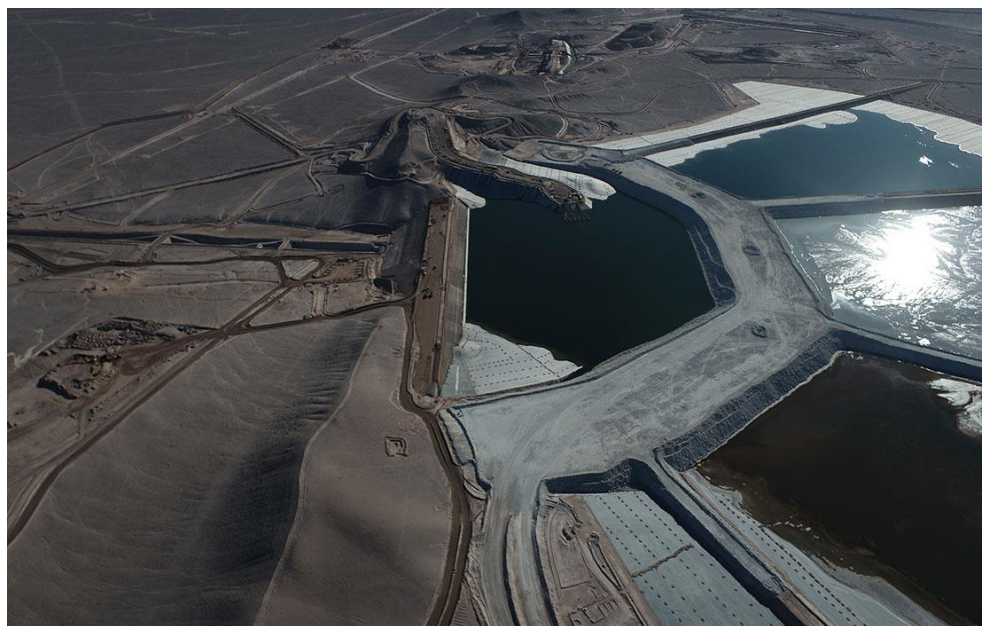
Figure 27. Supernatant Water Collected in Water Reservoir in Spence Tailings Storage Facility.
