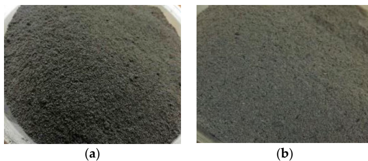
Figure 1. The shape of raw and processed SCBA. (a)—Raw SCBA. (b)—Processed SCBA.
