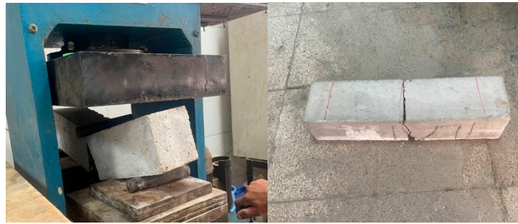
Figure 6. A typical flexure failure mode for raw and processed SCBA concrete specimens.
