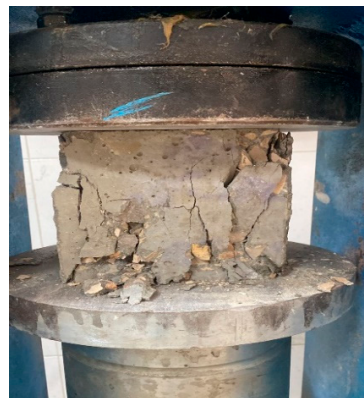
Figure 4. A typical compressive failure mode for raw and processed SCBA concrete specimens.
