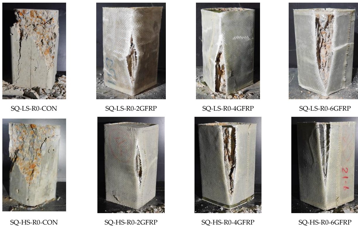
Figure 5. Ultimate failure modes of Group 1 specimens.
