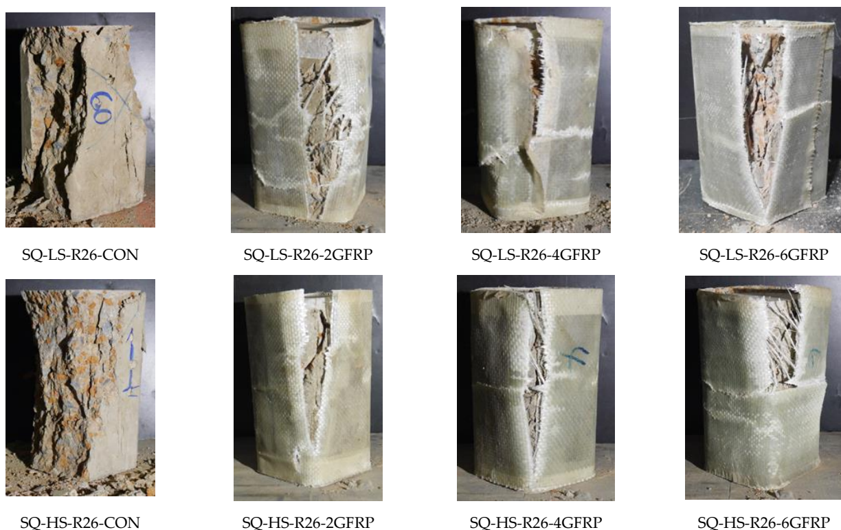
Figure 6. Ultimate failure modes of Group 2 specimens.
