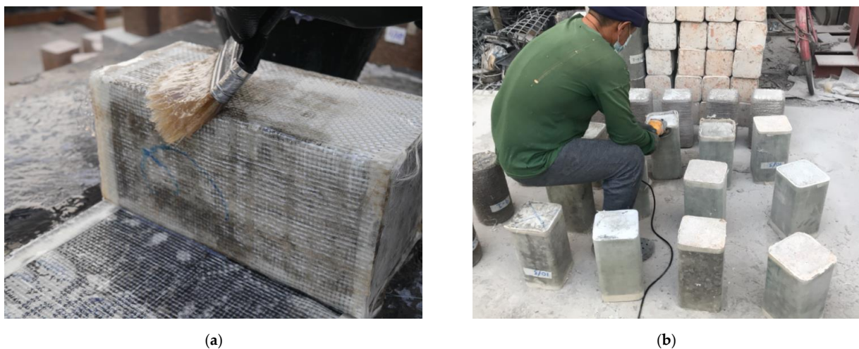
Figure 3. (a) Application of epoxy resin and (b) grinding of excessive GFRP portions and smoothing of the top and bottom surfaces.
