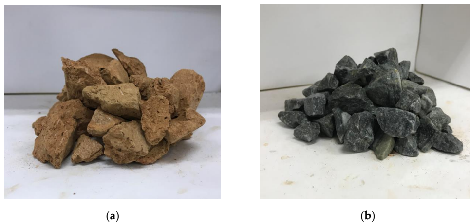
Figure 1. (a) Brick aggregates, and (b) natural aggregates.
