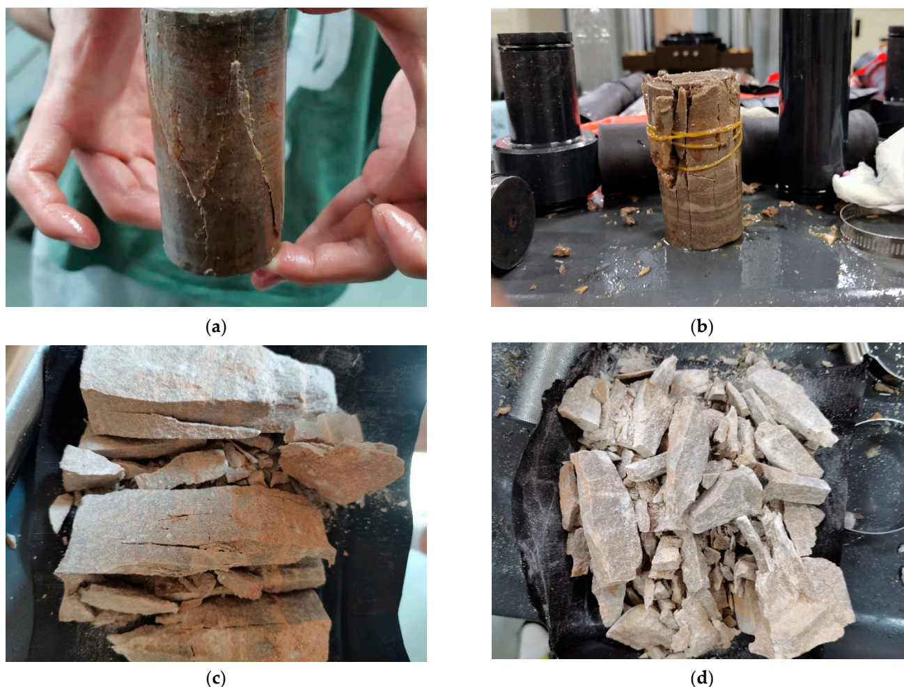
Figure 7. Characteristic morphology of the macroscopic destruction of rocks; (a) dissolution for 3 days; (b) dissolution for 7 days; (c) dissolution for 14 days; (d) dissolution for 21 days.
