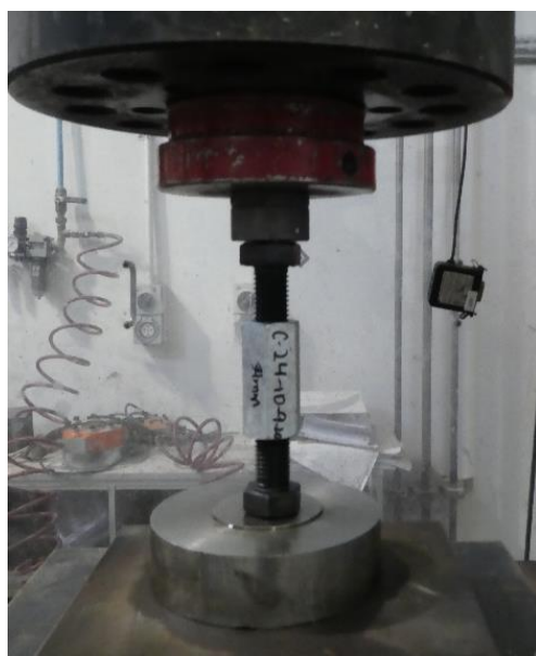
Figure 6. Test setup for coupling bolts under pure axial compression.
