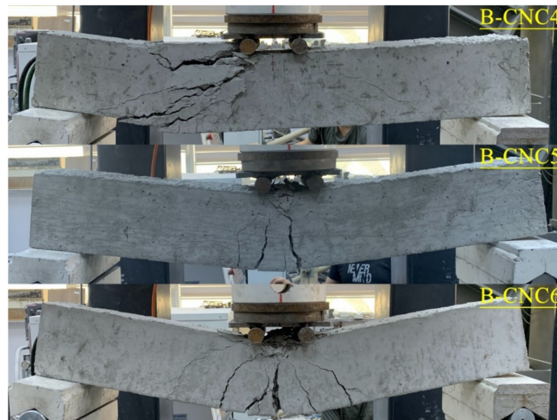
Figure 8. Failure and bending attitude of RCB for BCNC-4, BCNC-5, BCNC-6.
