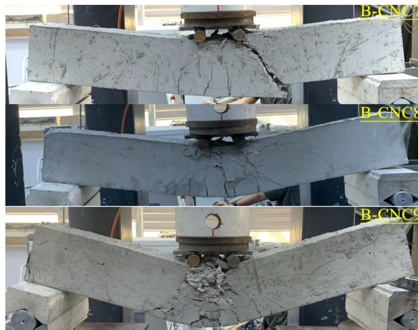
Figure 10. Failure and bending attitude of RCB for BCNC-7, BCNC-8, BCNC-9.
