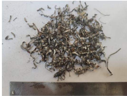
Figure 1. Waste steel scrap prepared for preparation of the concrete.
