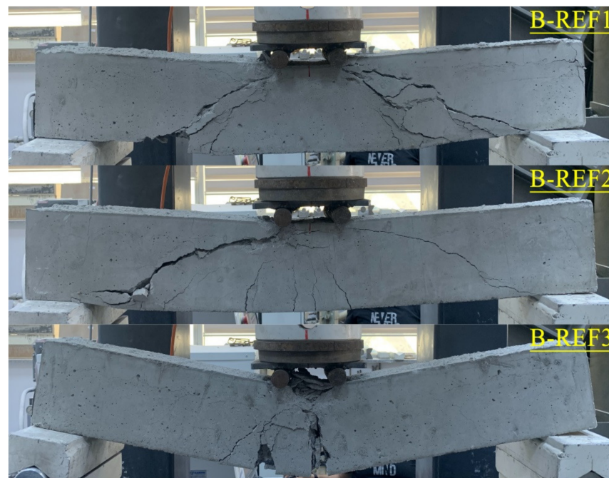
Figure 4. Failure and bending behavior of RCB for BREF-1, BREF-2 and BREF-3.
