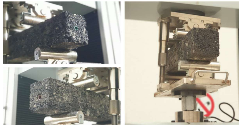
Figure 6. Three-point bending test conducted on asphalt specimens with and without geothermal pipes.
