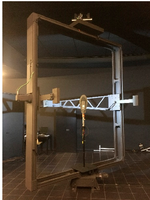
Figure 1. TechnoTeam Rigo 801 Near-Field Goniophotometer used to characterize the luminaire.
